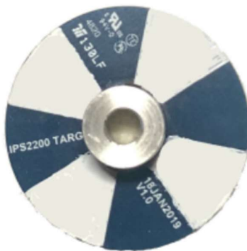
Figure 23. Reflector Board, Mounted onto Rotor
