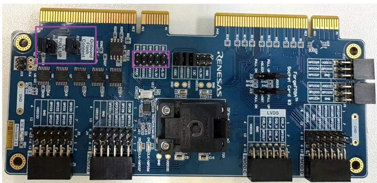
Figure 24. Jumpers and External Power Connection Points on the Board
