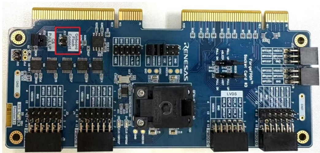
Figure 19. Disconnect Socket Card from Development Board and Remove the Jumper
