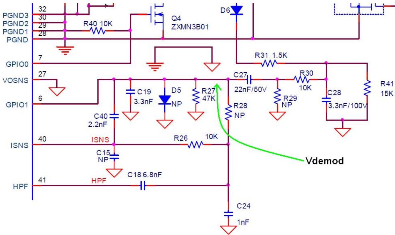
Figure 22. DEMODULATION most noise sensitive nodes, schematic highlight (Isns, HPF, Vdemod)
