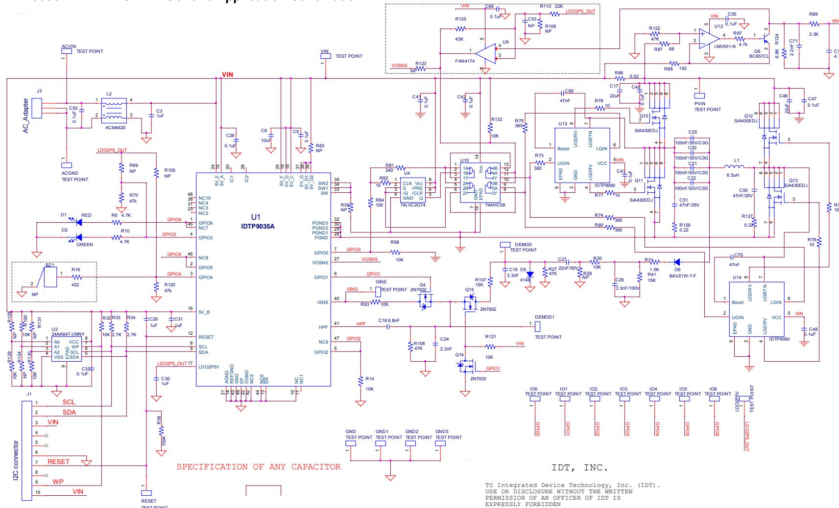
Figure 13. Complete IDTP9035A Application Schematic
