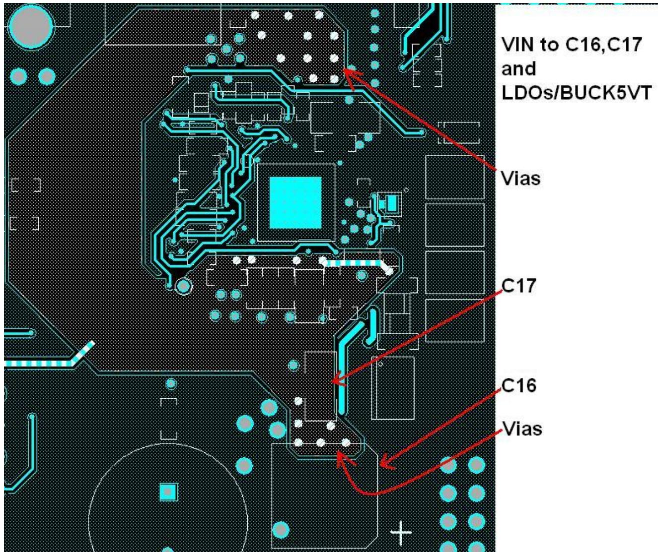
Figure 20. VIN route to C16, C17 and LDO/BUCK5VT caps on inner layer using many vias for layer transitions
