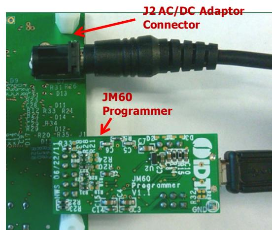
Figure 1. IDTP9035A-EVAL JM60, AC Adaptor connections. The AC/DC Adaptor plug and JM60 connectors are on the backside of the board. The AC Adaptor must be set to 5V for proper operation.
