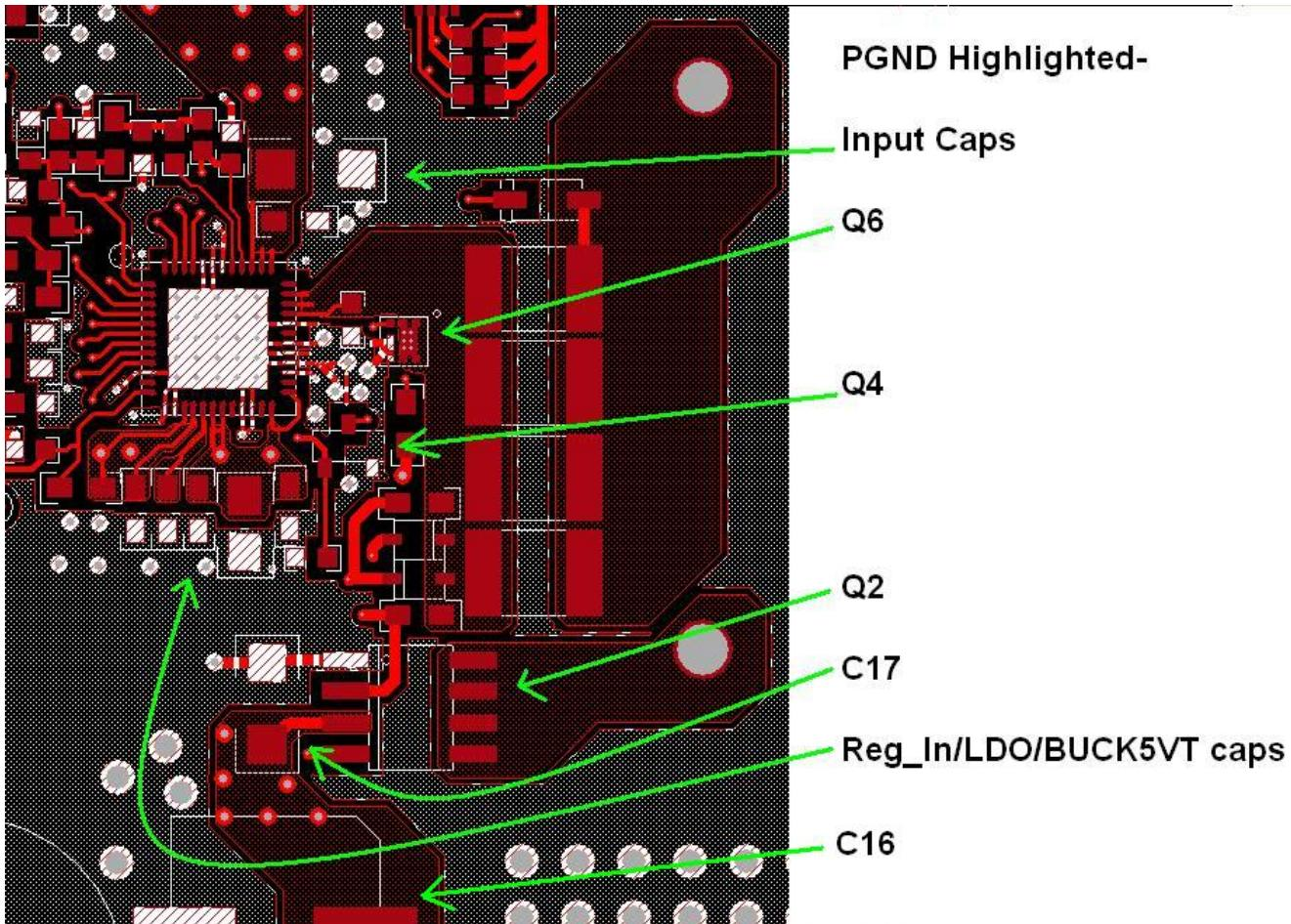
Figure 19. PGND routing and component placement.
