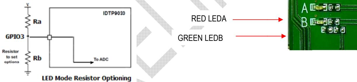
Figure 8. IDTP9035A LED Resistor Options. The IDTP9035A LED indicators are connected to GPIO0, 3. Currently only LEDA and LEDB are operational and only Green LEDB contains the resistor options.
