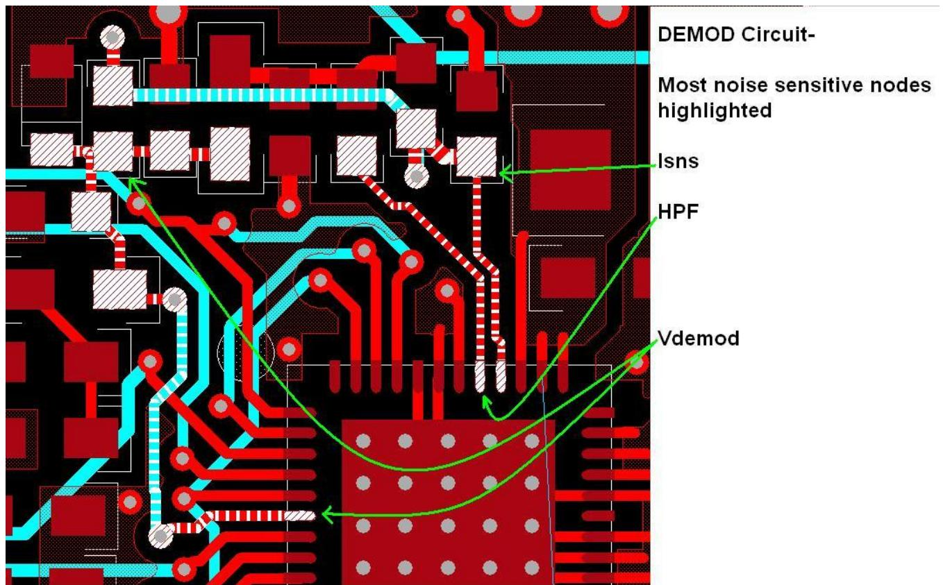
Figure 21. DEMODULATION most noise sensitive nodes, placement routing recommendations
