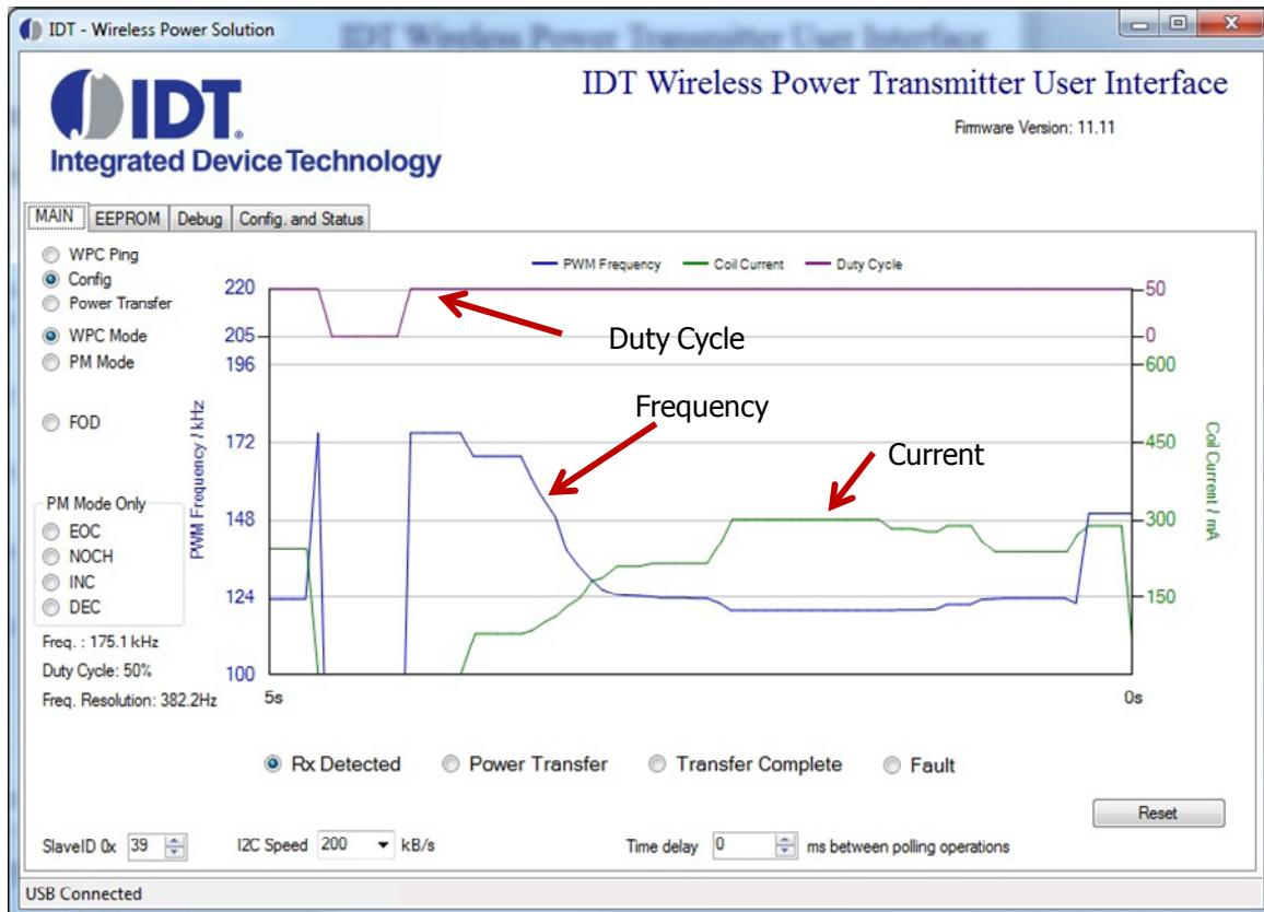
Figure 4. Windows GUI MAIN Tab Details and Signals.
