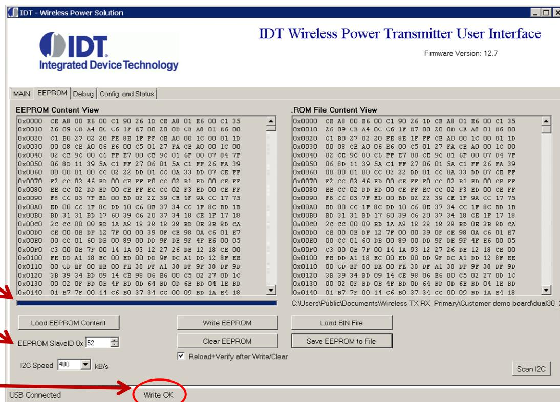
Figure 7. After Loading a BIN File and Writing to the EEPROM.
