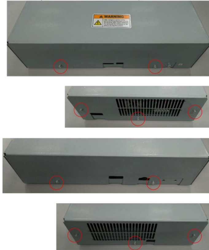
Fig. 3-1 Removing the main body cover
