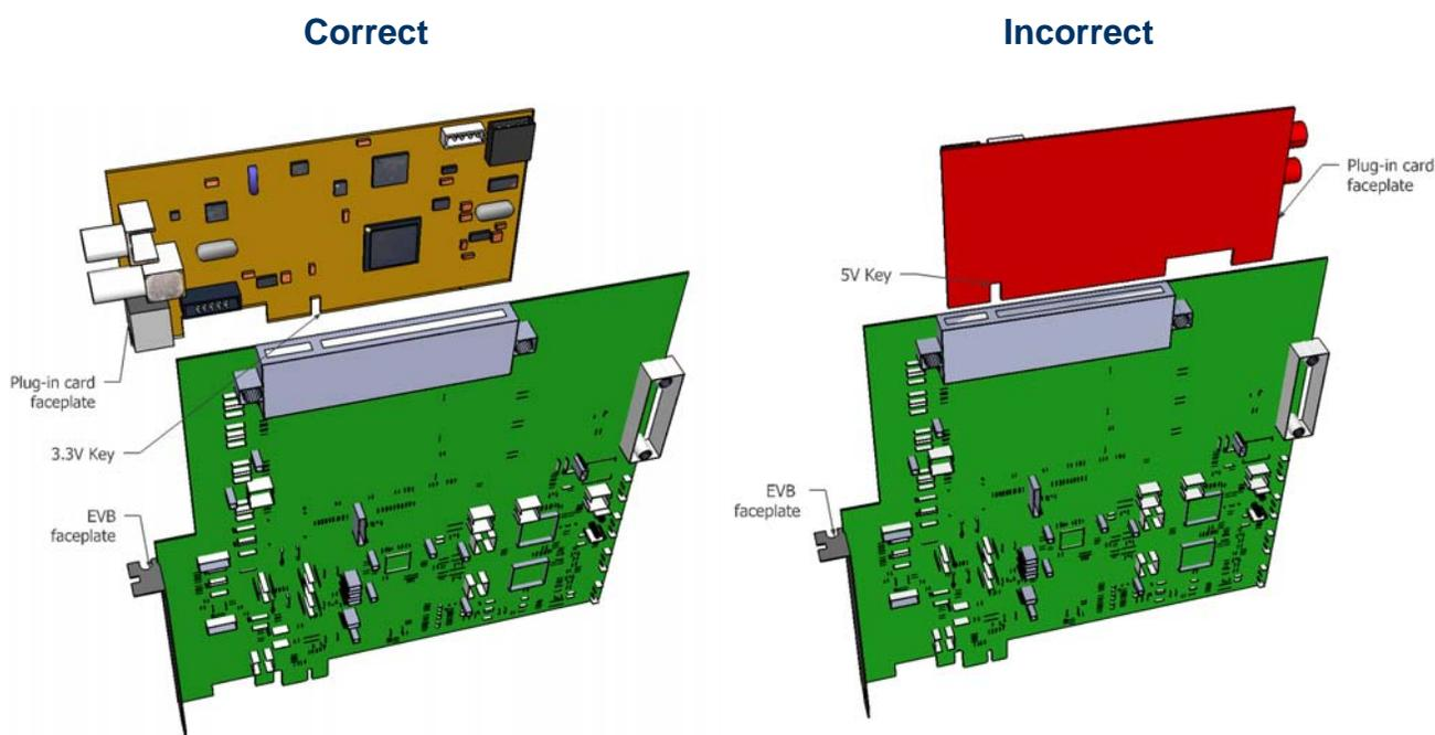
2. Do not use a keying adaptor to connect a 5V keyed card on the evaluation board unless the evaluation board has been modified for 5V operation (see the following diagram).
