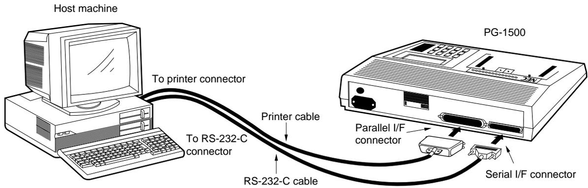
**Figure 2-2. Connections of Serial I/F (RS-232-C)**
