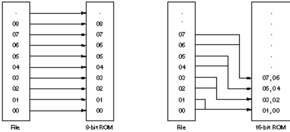
Figure 4-3. In the Case of “16-Bit 2-Partition” (BE, BO)
