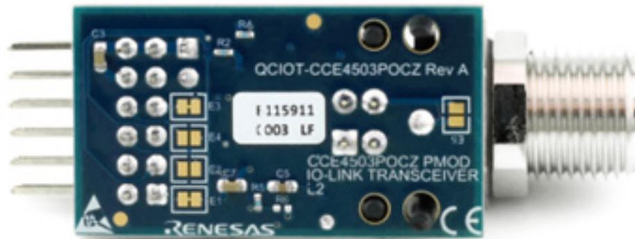
Figure 5. QCIOT-5 IO-Link Device Transceiver Board (Bottom)
