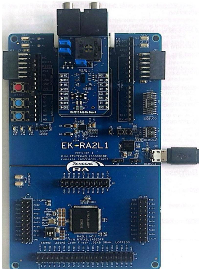
Figure 3. QCIOT-DA7212EVZ Click Board with EK-RA2L1 MCU
