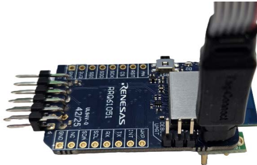
Figure 14. J-Link Connection Using Tag-Connect Needle Adapter
