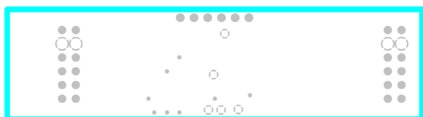
Figure 11. Internal Plane-1 (GND)
