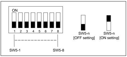
Figure 3.2 Setting the 8-bit DIP Switch
