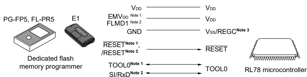
Figure 28-2. Communication with Dedicated Flash Memory Programmer
