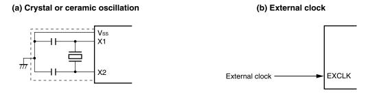
Caution When using the X1 oscillator, wire as follows in the area enclosed by the broken lines in the Figure 5-19 to avoid an adverse effect from wiring capacitance.
