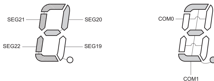
Figure 16-27. Two-Time-Slice LCD Display Pattern and Electrode Connections (e.g. the fourth digit in Figure 16-28)
