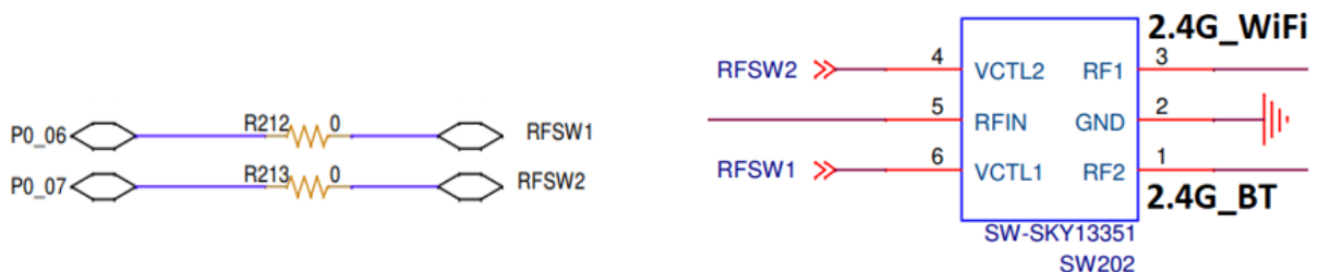
Figure 75. RF SPDT switch circuitry of RA6W2 daughterboard
