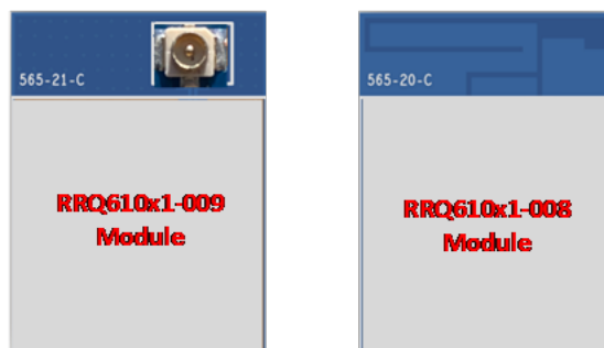
Figure 76. RRQ610x1-009 uFL (left) and RRQ610x1-008 printed antenna (right)
