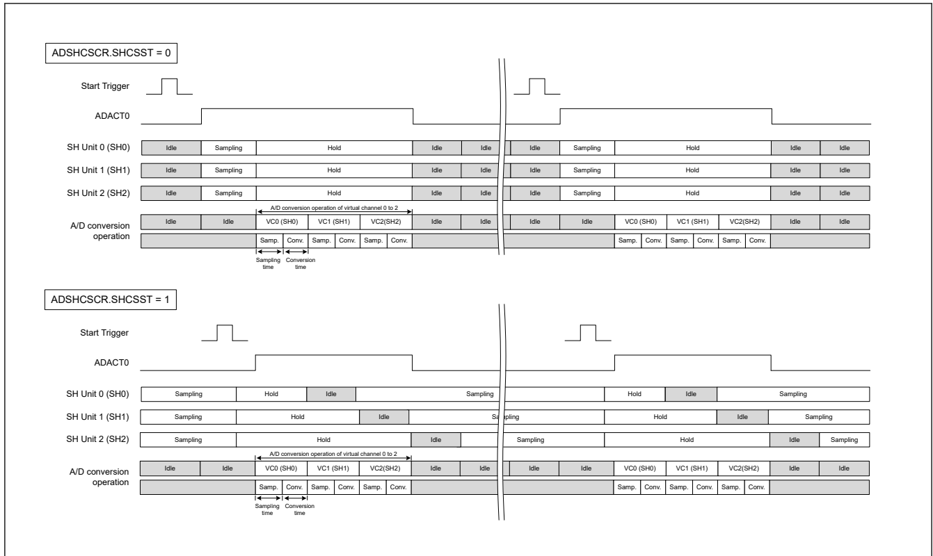
Figure 53.23 Difference between the function of channel-dedicated sample-and-hold circuit when using or not using constant sampling
