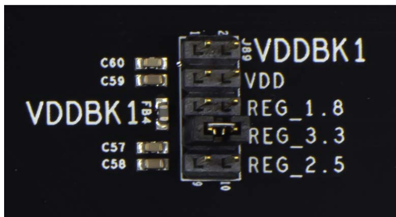
Figure 14. Power Source Selection for BANK Voltage
