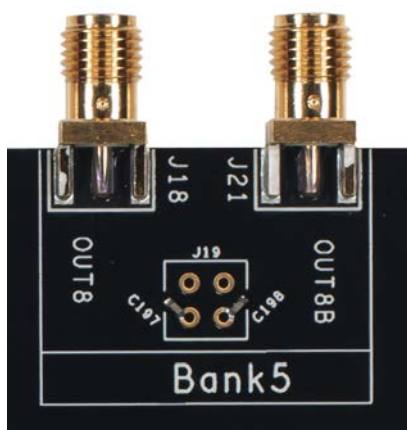
Figure 10. Output Termination with SMA Connector, Top Side
