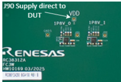
Figure 7. J90 Board Input
