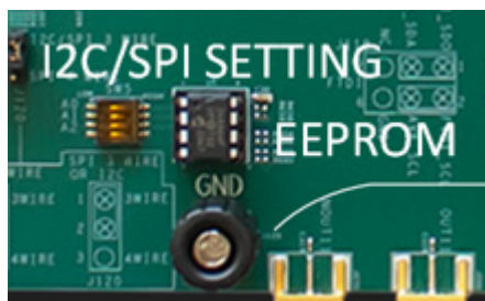
Figure 20. EEPROM in Socket
