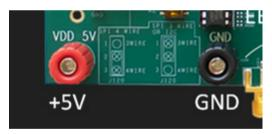
Figure 5. External 5V Board Input
