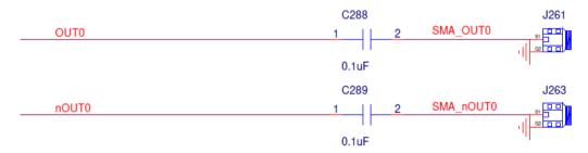
Figure 18. Output Clock AC-Coupling
