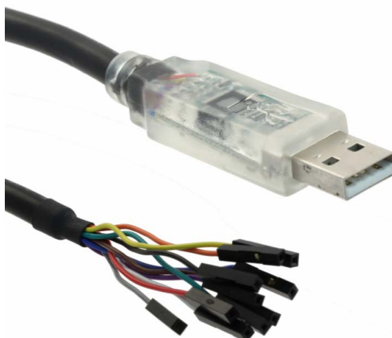
Figure 6. FTDI Dongle: USB Type-A at PC end and 10 free-wires at the other end
