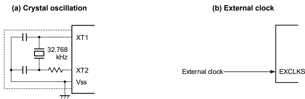
Figure 5-22. Example of External Circuit of XT1 Oscillator
