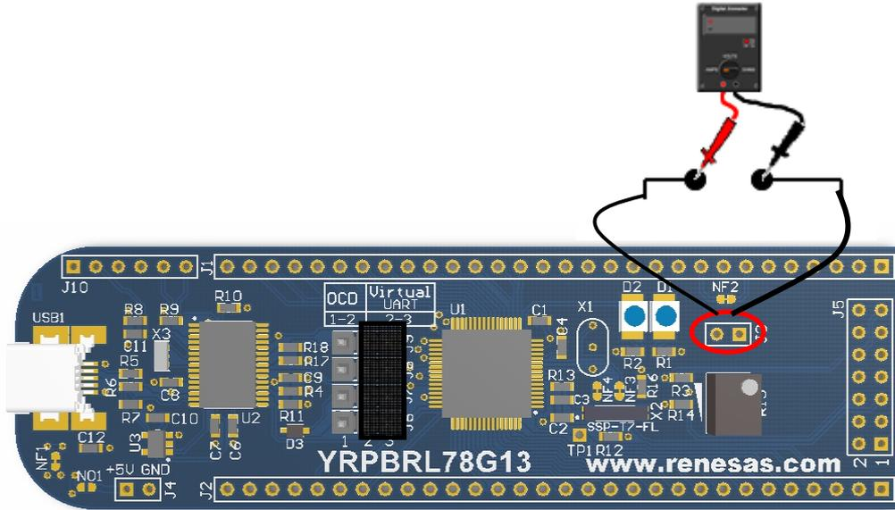
Figure 52: Multi-Meter Connection for Current Measurement
