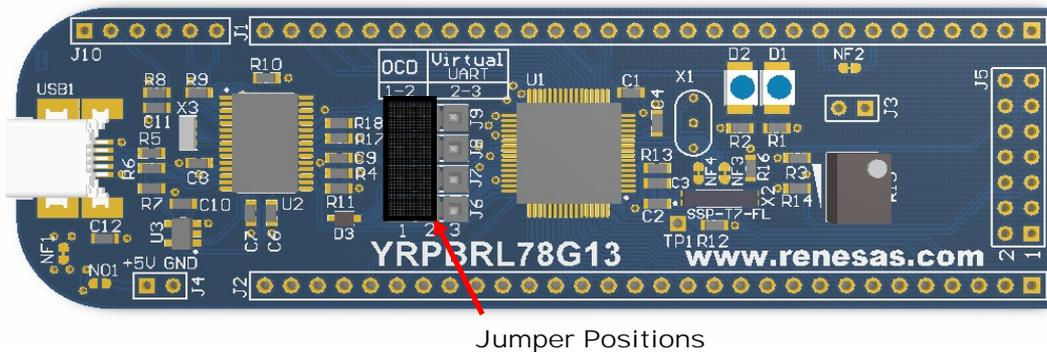
Figure 22: Stick in Flash Programming Configuration
