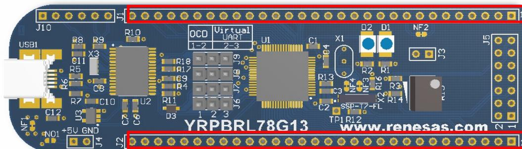
Figure 5: External Connectors J1 and J2
