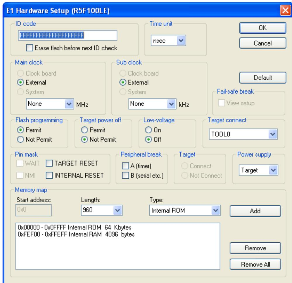
Figure 43: E1 Emulator Hardware Setup for TOOL0 Interface
