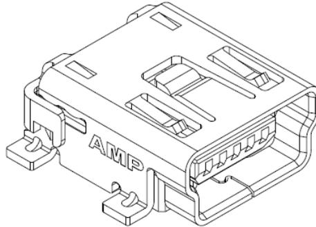
Figure 4: Connector USB1, Mini USB B Type Connector Pin Configuration
