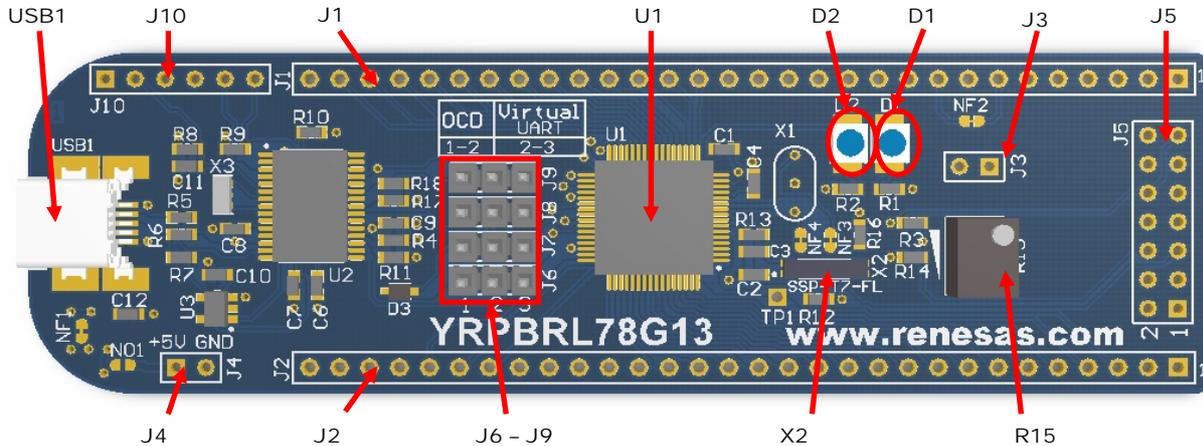
Figure 2: YRPBRL78G13 Board Components
