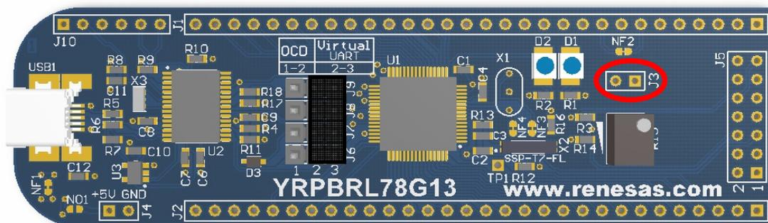
Figure 44: Current Measurement Connector
