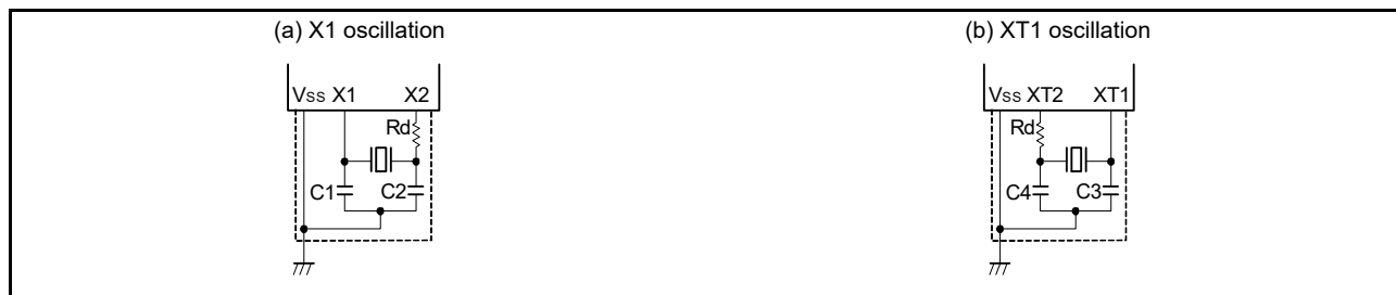
Figure 6 - 23 Examples of External Circuits
