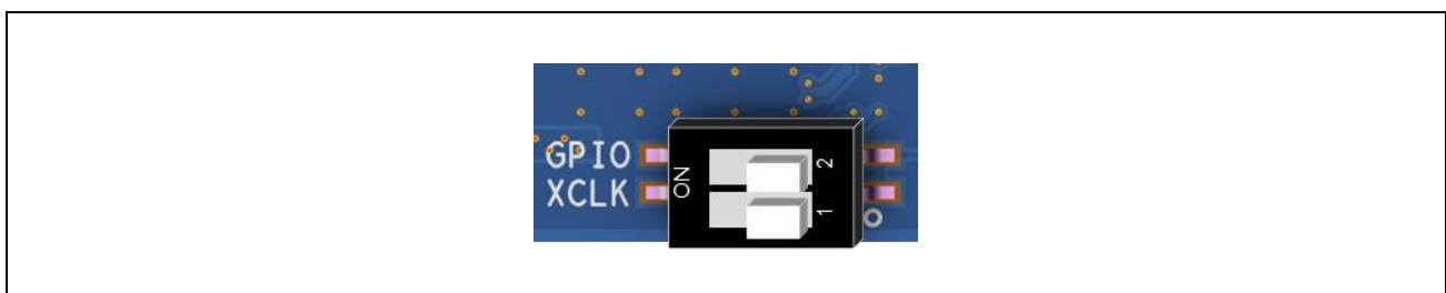
Figure 3.4 (b) The Location and the Default Setting of SW1
