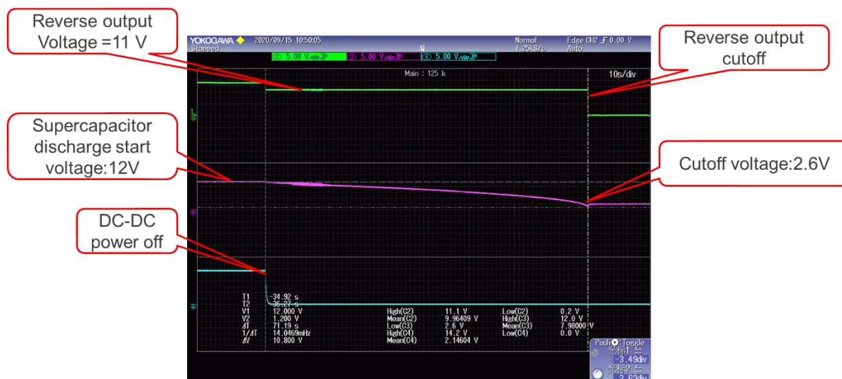
Figure 7 Discharging in CC Mode(200mA)
