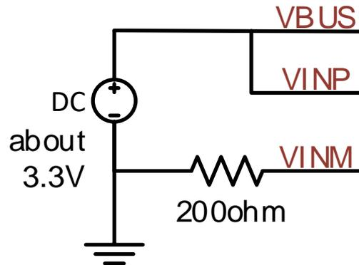
Figure 2-1 Current Measurement Circuit Example
