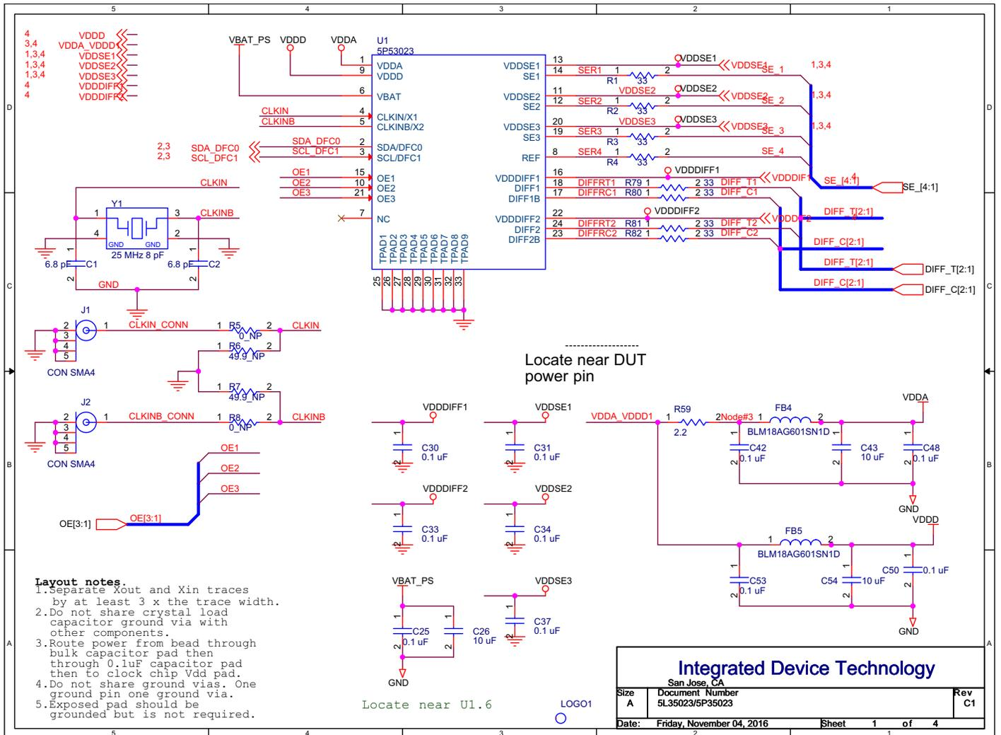
Figure 6. Evaluation Board Schematic (2)
