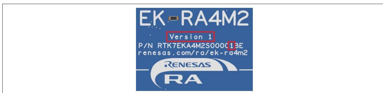
Figure 5. Identification of the Kit Version Number on the EK-RA4M2 Board
