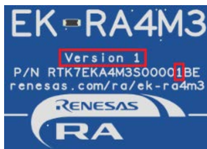
Figure 5. Identification of the Kit Version Number on the EK-RA4M3 Board
