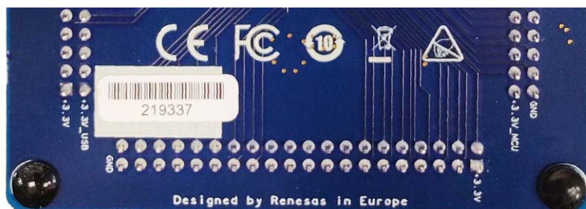
Figure 7. Identification of the Serial Number on the EK-RA4M3 Board
