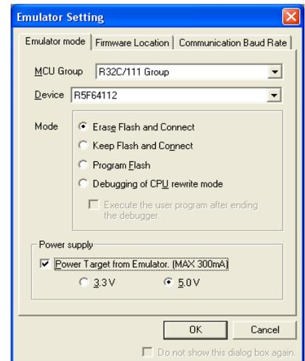
31. Please check the option "Erase Flash and Connect" Select the option "Power Target from Emulator" and select radio button "5.0V".
