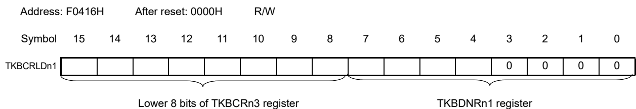
Figure 10 - 16 Format of 16-bit Timer KB Compare 3L & Dithering Count Register n1 (TKBCRLDn1)
