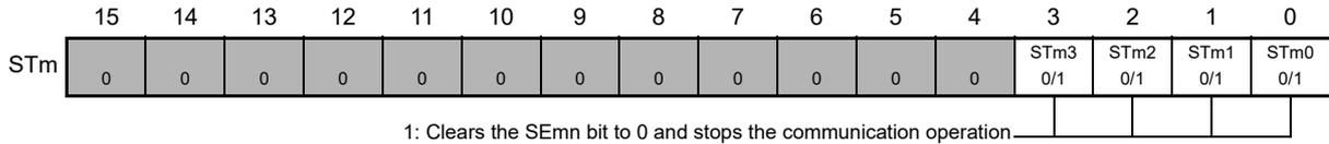
\* Because the STmn bit is a trigger bit, it is cleared immediately when SEmn = 0.
