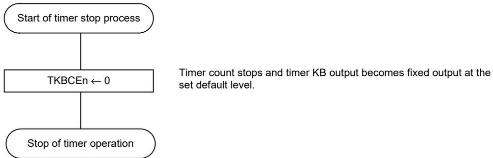
**Figure 10 - 24 Timer KB Operation Setting Example (Compare Register Batch Overwrite Flow)**
