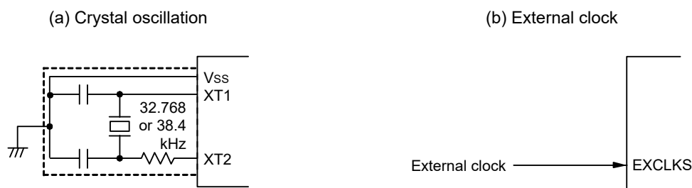
Figure 6-21. Example of External Circuit of XT1 Oscillator
