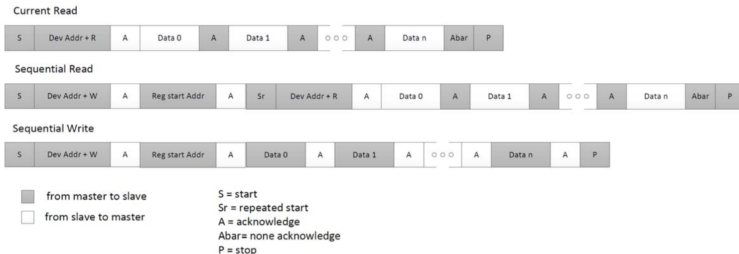
Figure 2. I 2 C R/W Sequence
