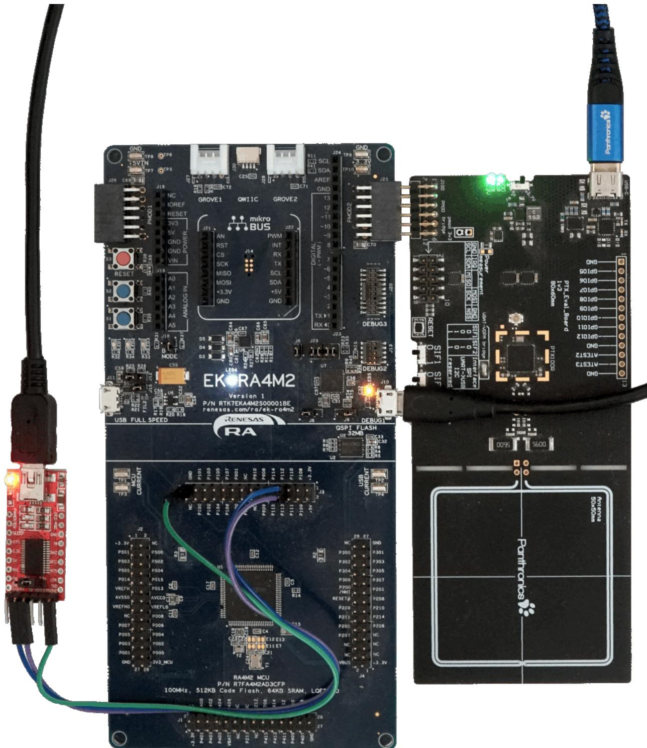
Before powering up from the USB-C port, it is important to remove the jumper "pmod 3v3 bridge" and set both of the **SIF1** and **SIF2** switches on the PTX100R evaluation board to "**0**" state to select the SPI communication protocol.
