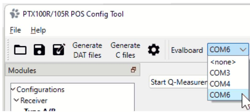
The config tool is using the hardware flow control functionality of the UART by default, which is not provided in this case. As a result, the **tunneling mode** should be enabled in the **File > Settings** menu.
