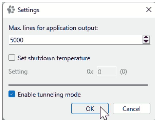
The configuration is ready; any config tool application (for example, Q-Measurement) started will now communicate with the PTX100R via the tunneling firmware.
