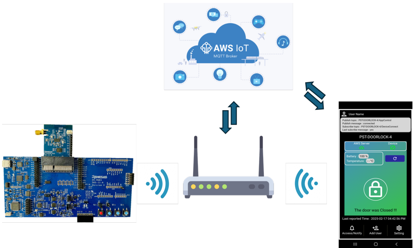
Figure 1. Architecture of AWS IoT reference application
