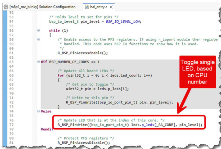
Figure 93: Multicore Blinky - Updated Code
