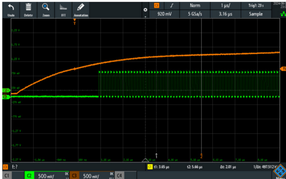
Figure 37. Continuous 7.68MHz Pulse (Green) with GPIO Dip Switch Trigger (Orange)
