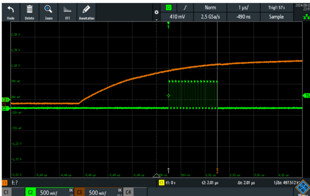
Figure 35. Single Pulse Train (0x10 Pulses) (7.68MHz (Green) and GPIO Trigger (Orange))
