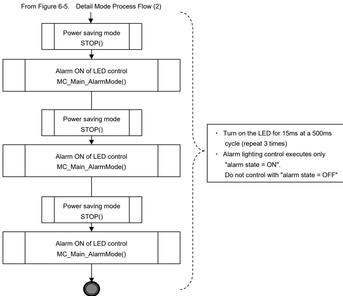
Figure 6-6. Detail Mode Process Flow (3)
