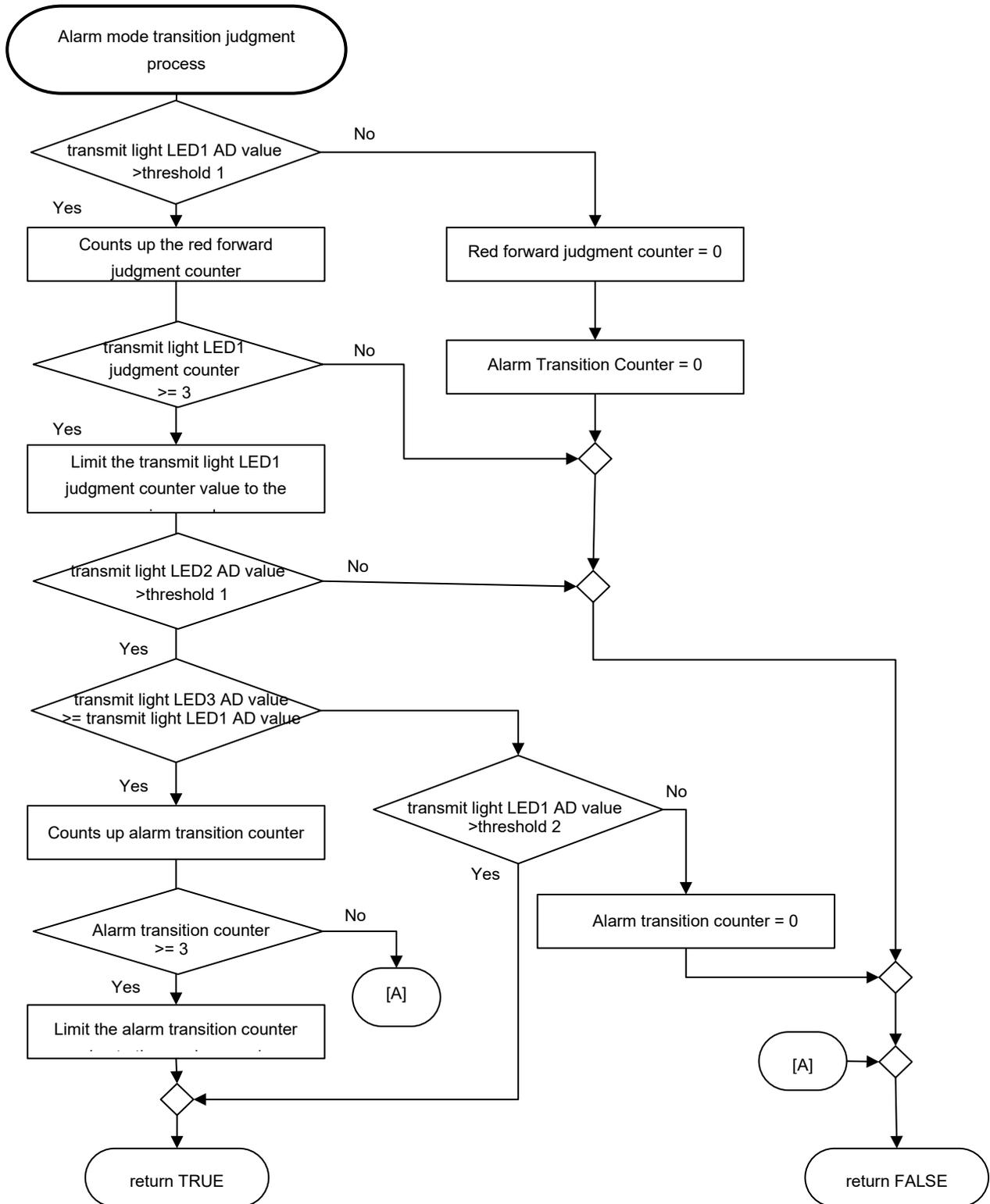
Figure 6-7. Alarm Mode Transition Judgment Process Flow
