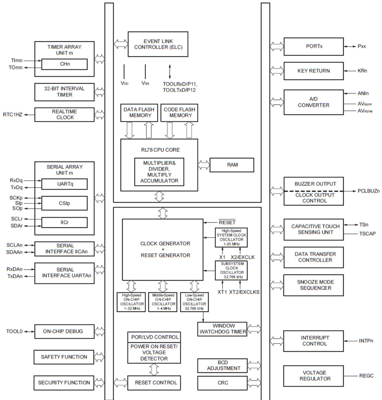
Figure 3-2. RL78/G22 Block Diagram
