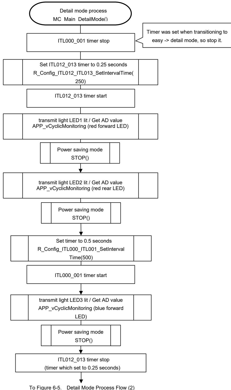
**Figure 6-4. Detail Mode Process Flow (1)**
