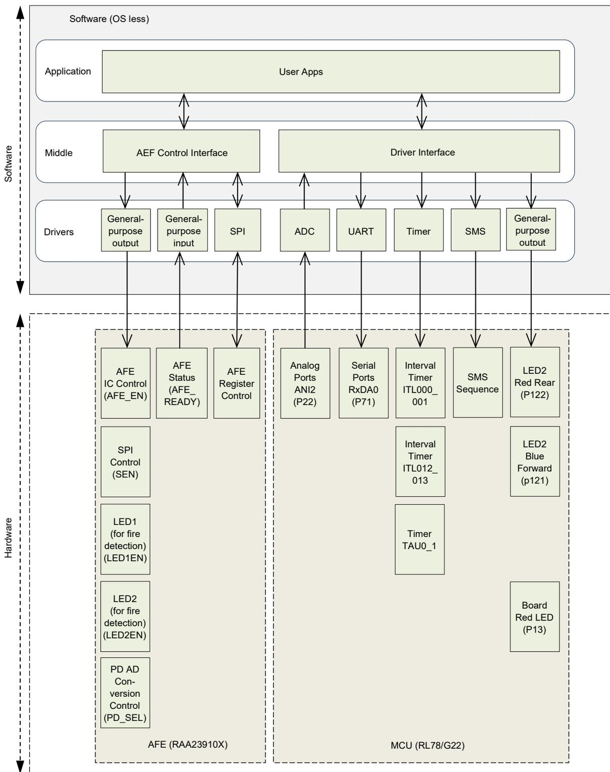
Figure 4-1. Software Configuration
