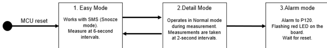
Figure 5-1. State Transition Diagram
