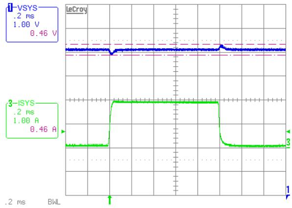
**Figure 25. Reverse Mode, 20VADP, 12VSY, 0-2A Transient Load**
