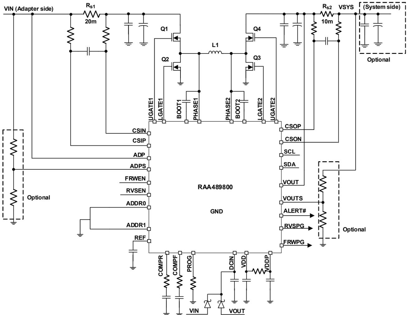
Figure 1. Block Diagram
