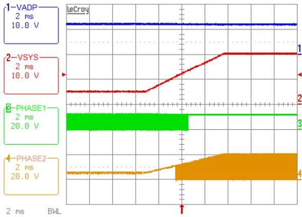
Figure 14. VSYS Voltage Ramps Up in Forward Mode, Buck -> Buck-Boost -> Boost Operation Mode Transition
