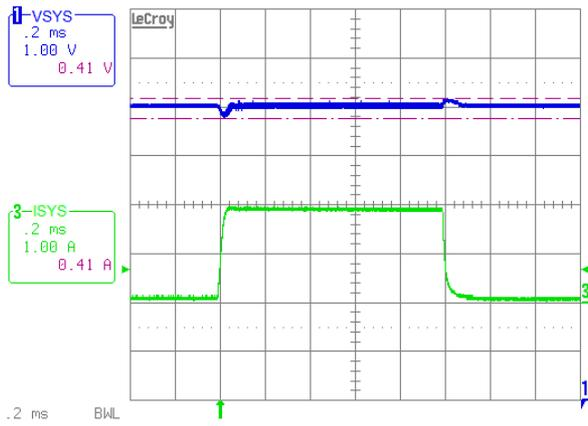
**Figure 24. Forward Mode, 5VADP, 12VSY, 0-2A Transient Load**
