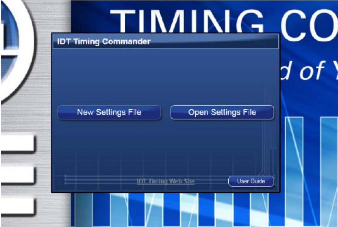
A settings file (.tcs) is a text file where the device input and output requirements are stored. From this window, an existing setting file can be opened to restore a configuration, or a new setting file can be created.
