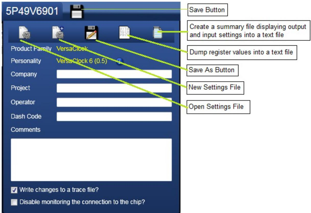
8. **Save the Settings File** – After the configuration is complete, click on the disk symbol at the upper left corner to save the setting file, as shown below.
