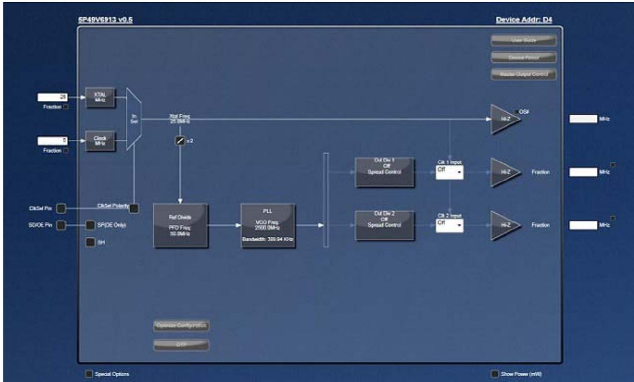
As shown in Figure 20, the Timing Commander window looks a lot like the 5P49V6901 device window, all buttons and functionality are identical - the only difference is the number of outputs.
