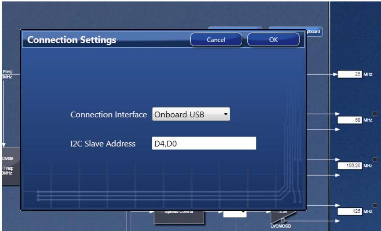
Use the default values in Connection Settings window and click OK to close it. Then click the chip symbol in the corner to bring out read/write command. When the connection is functioning, the area will turn green with “read” or “write” indicators. See Figure 15. The arrow pointing out of the chip means “reading from the chip”; the arrow pointing into the chip means “writing to the chip”.
