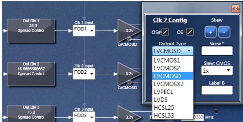
Clicking on the triangle box brings about output frequency configurations: Output type, Slew rate, Output voltage and Skew.
