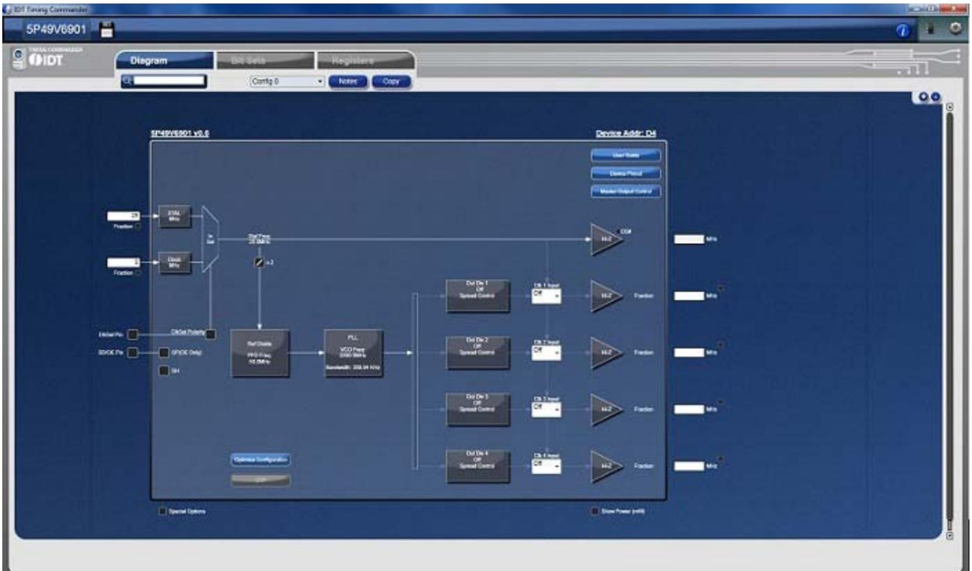
In the above configuration window, input source and frequencies can be selected and entered. The GUI will automatically configure the PLL to generate desired outputs, based on the Reference divider and Feedback Divider settings.
