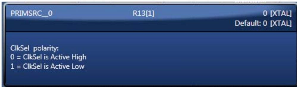
The CLKSelPol check box needs to be checked if using the CLK is selected as primary source and if CLK sel pin low like in Figure 5b. The timing commander will display the selected source based on the selection. The En\_Buff box will be then enabled.
