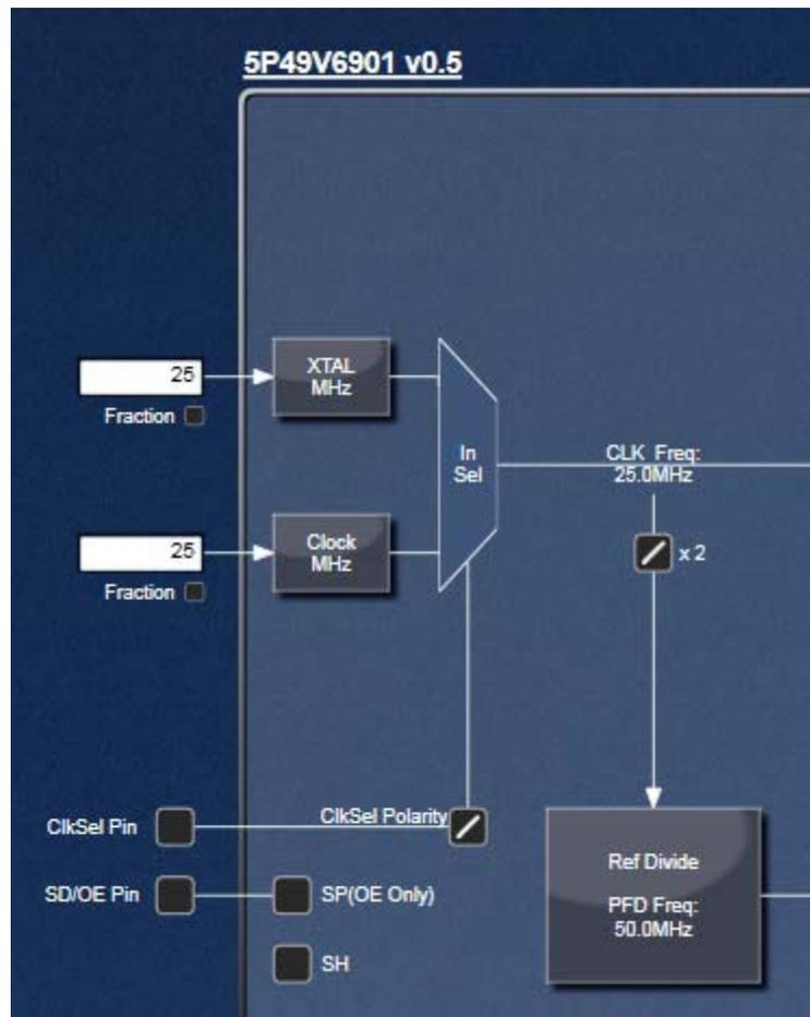
**5. Input Frequency Fraction box** -- Input clock can be entered as a fraction if fraction box is checked and Fraction word is clicked as shown in figured 5c below. The calculation button will give the final frequency that will be entered in the input box. The fraction can be used for both Xtal and CLKIn inputs.
