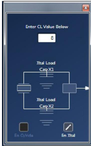
The max CL that can be created in the IC is 11.4pF. When entering a larger value, Timing Commander will display a window advising how much capacitance to add externally to each crystal pin to achieve the desired CL value (see Figure 6). TC is rounding the values to a integer value for the advisable external capacitors.
