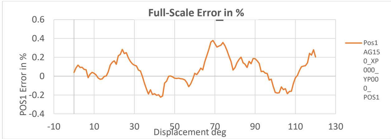
Figure 4. Accuracy with Linearization at 1.5mm Airgap (AG150)
