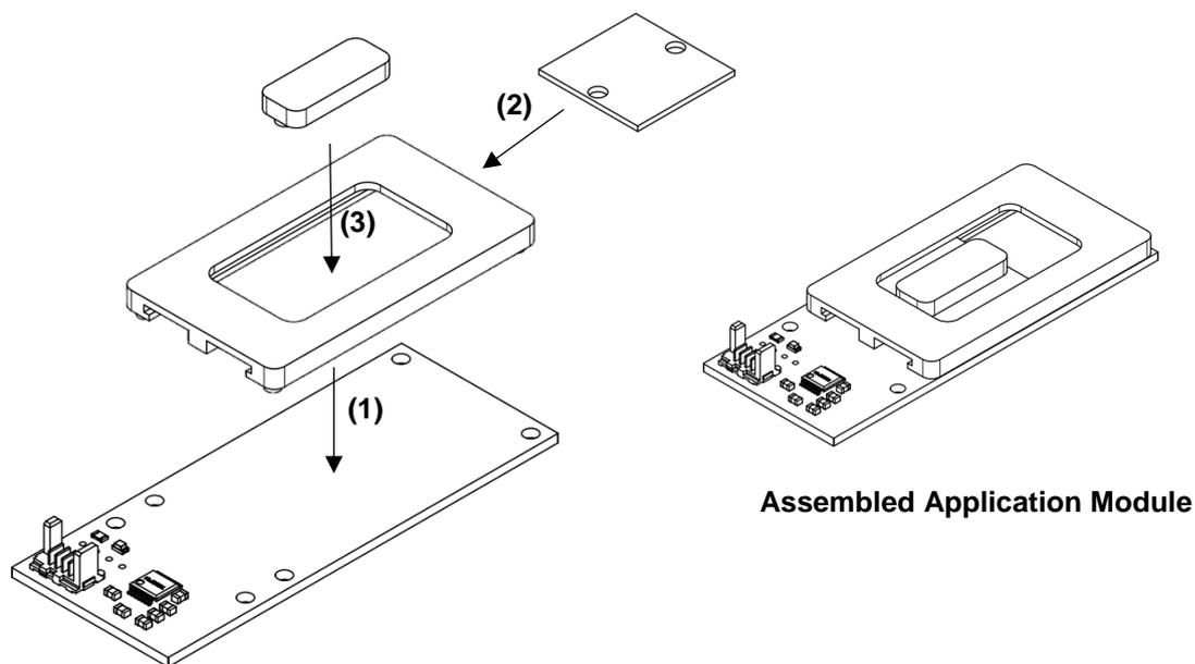
Figure 2. Target Holder Assembly
