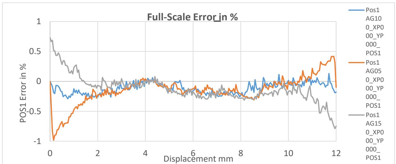
Note: AG050 = 0.5mm airgap; AG100 = 1mm airgap; and AG150 = 1.5mm.
