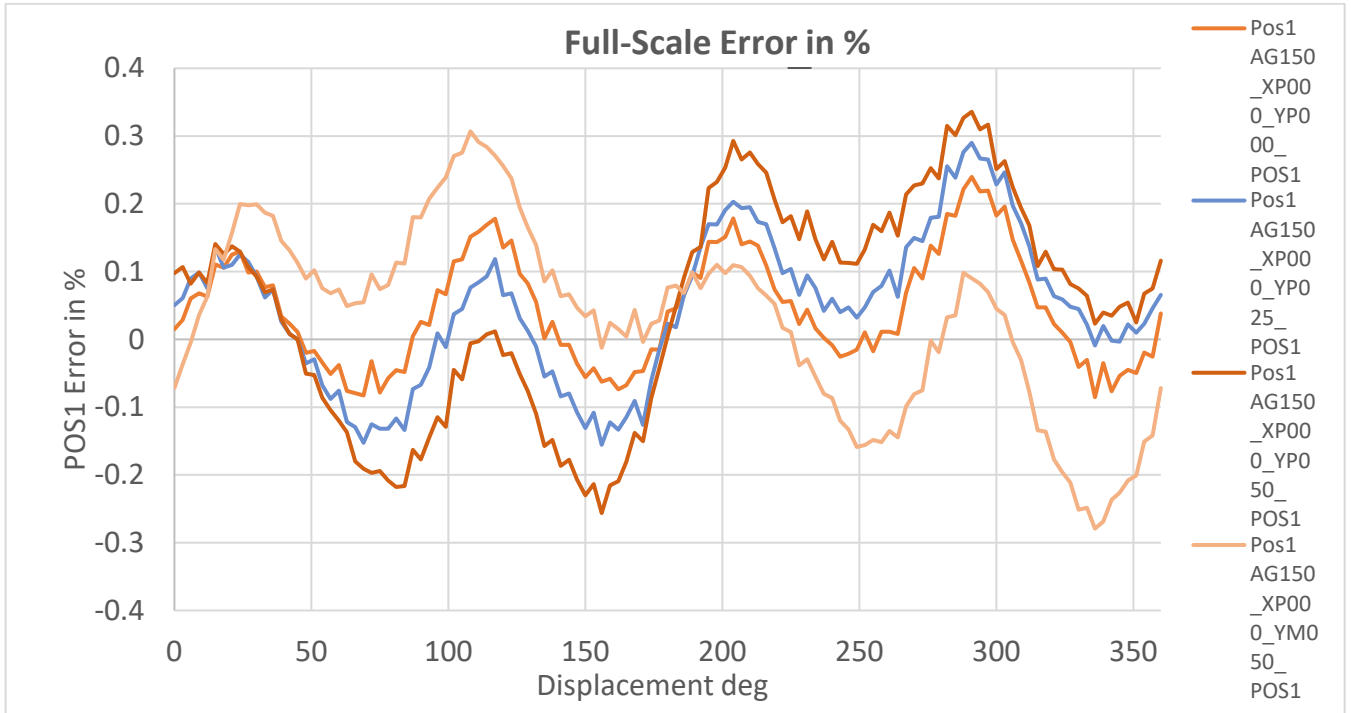
Figure 6. Accuracy with Linearization at 1.5mm Airgap and Effects of Displacement in Y
