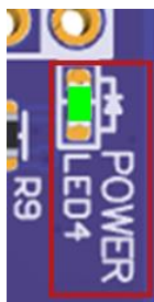
Figure 18. Power LED (FPB-RA2T1 Top View)
