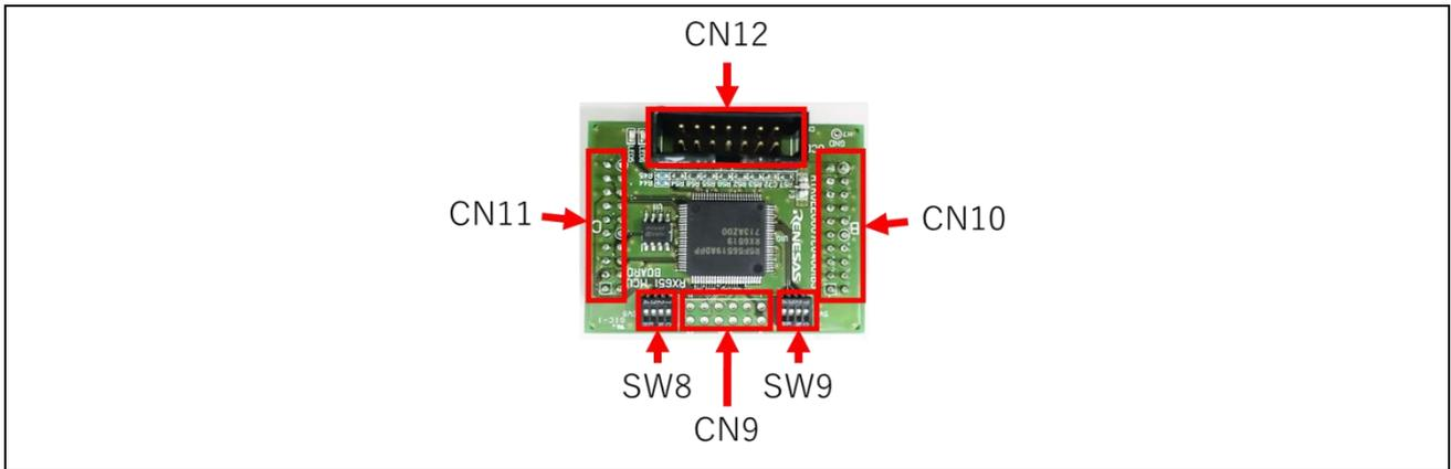
**Figure 1-9 RX651 MCU board connector and SW**
