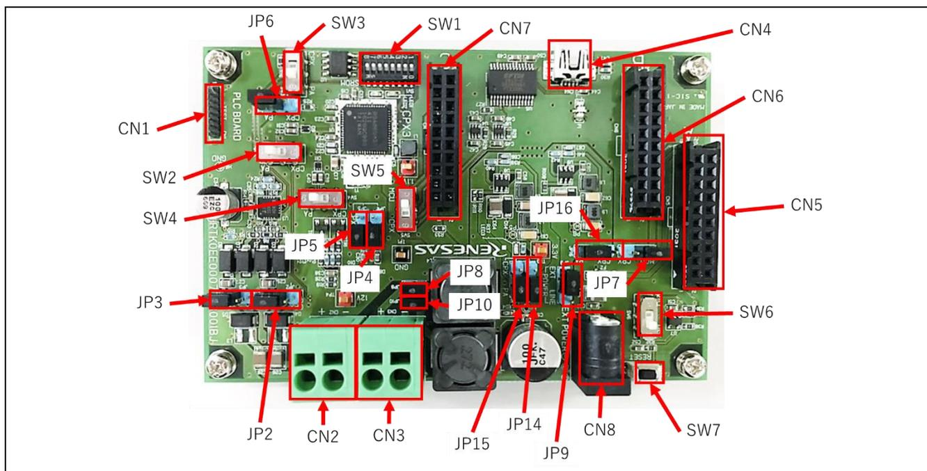
Figure 1-8 PLC board connector, JP, and SW
