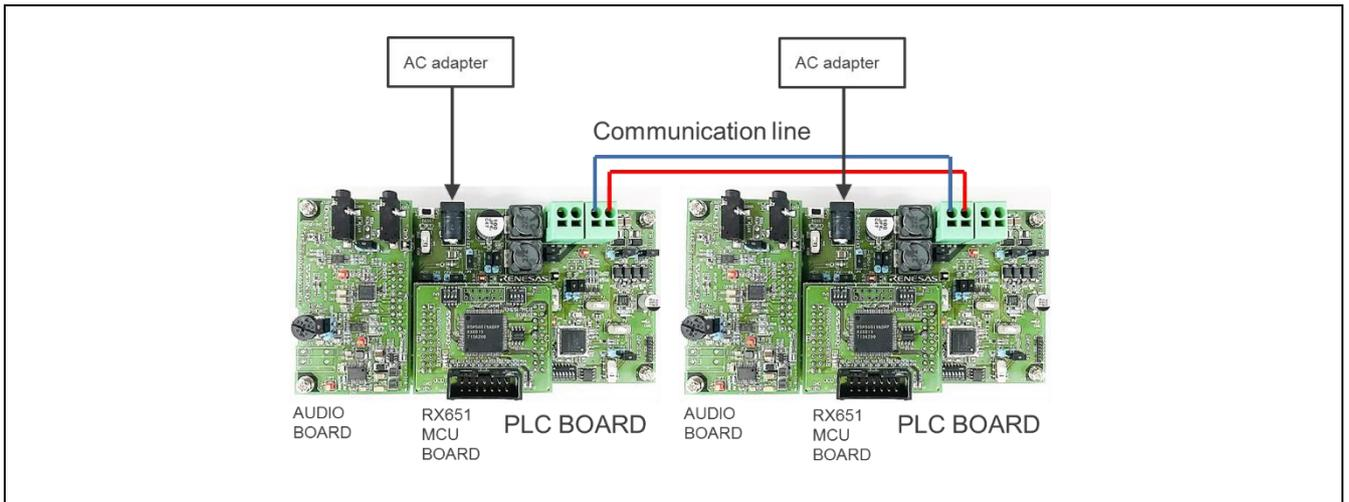
**Figure 2-6 Condition 5 : PLC board + RX651 MCU board + Audio board**
