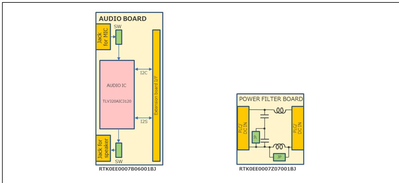
Figure 1-7 Audio board, Power Filter Board Function block diagram
