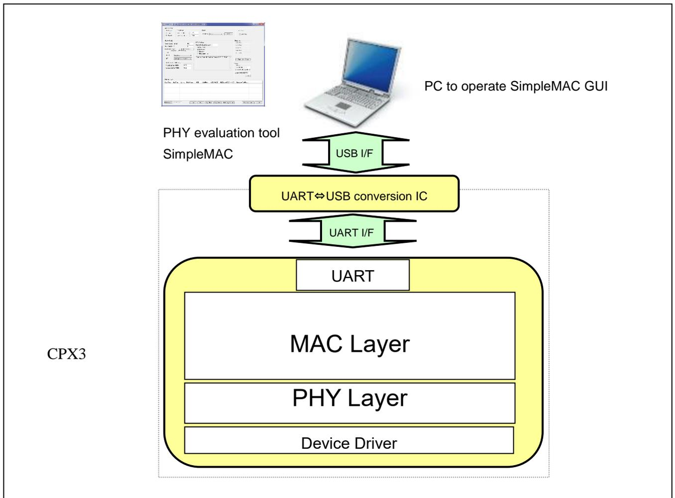
Figure 1-5 PLC evaluation software configuration
