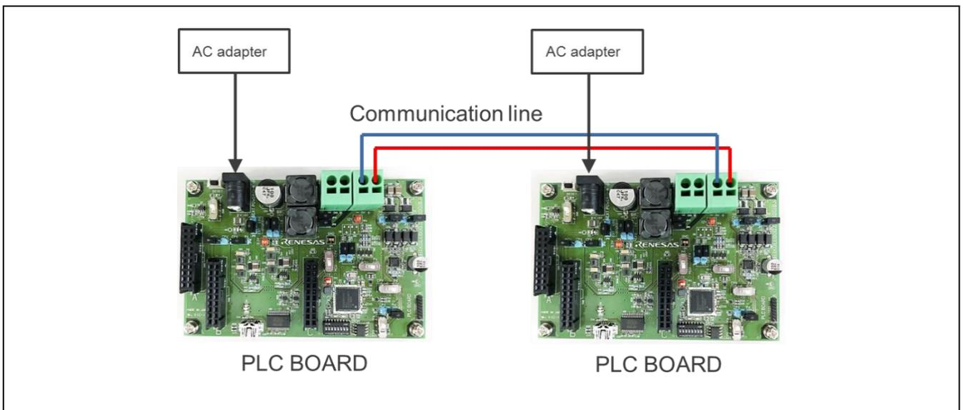
Figure 2-3 Condition 2: PC board connection example of DC power supply from the AC adaptor (1)
