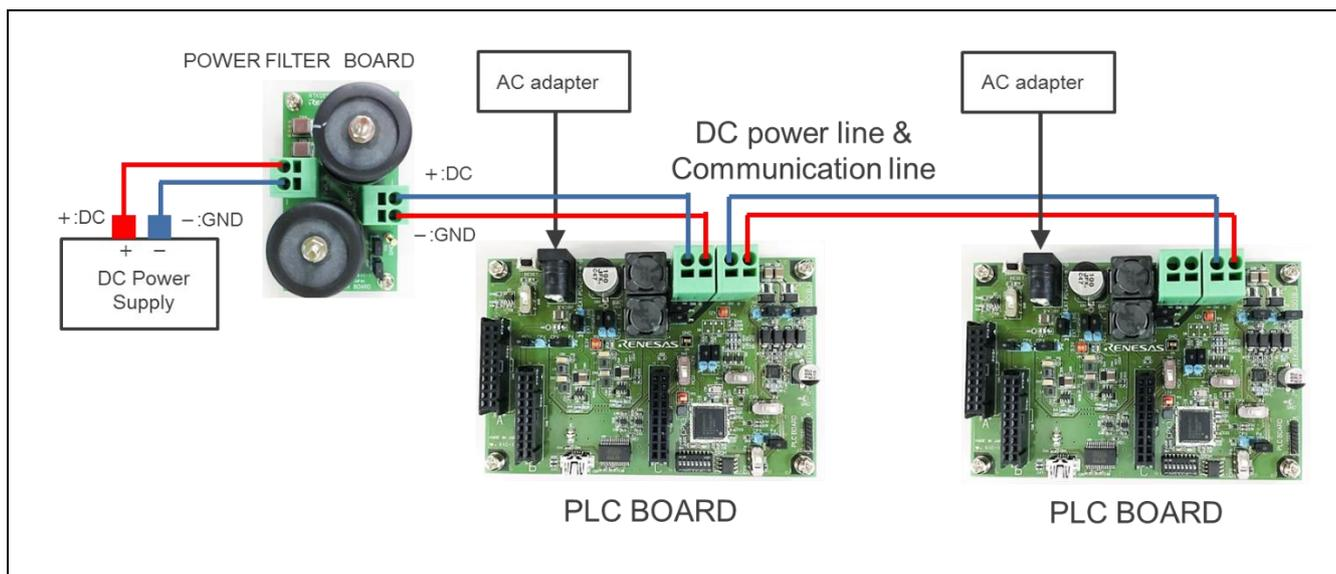
Figure 2-4 Condition 3: PC board connection example of DC power supply from the AC adaptor (2)
