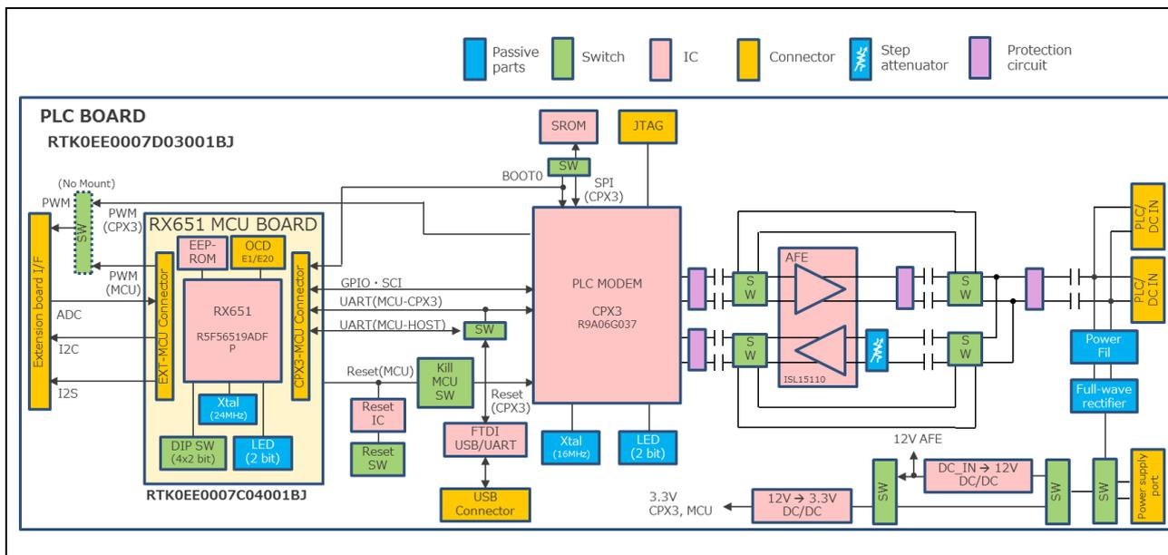
Figure 1-6 PLC board, RX651 MCU board Function block diagram
