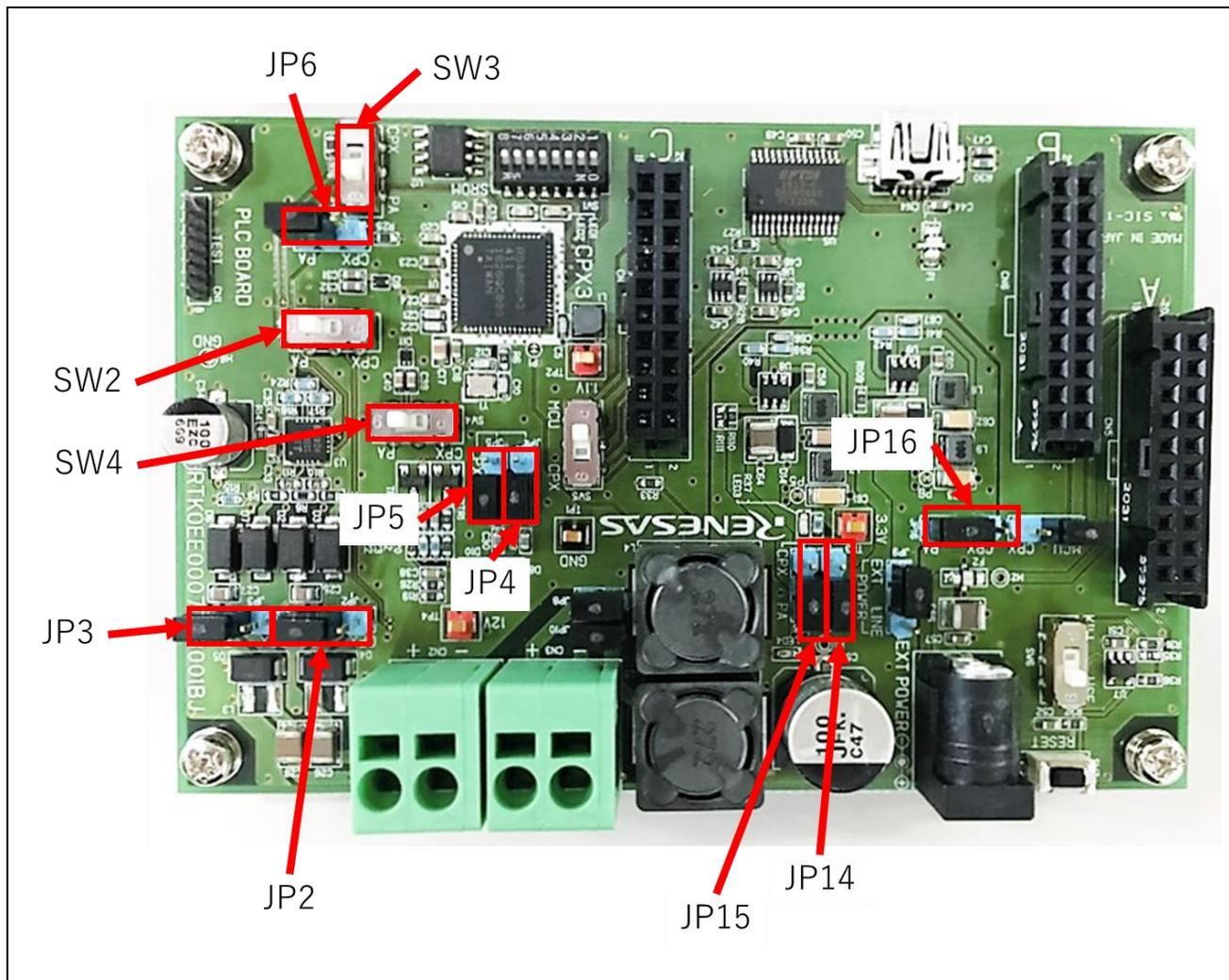
Figure 3-1 Parts used for switching drive system
