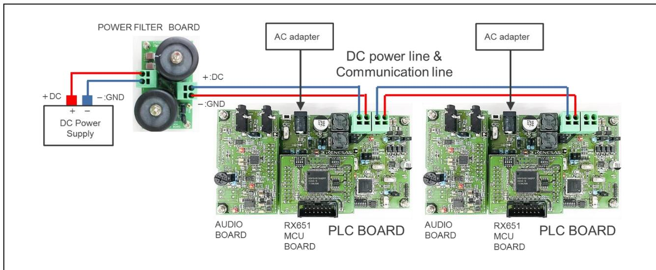
Figure 2-5 Condition 4: PLC board + RX651 MCU board + Audio board
