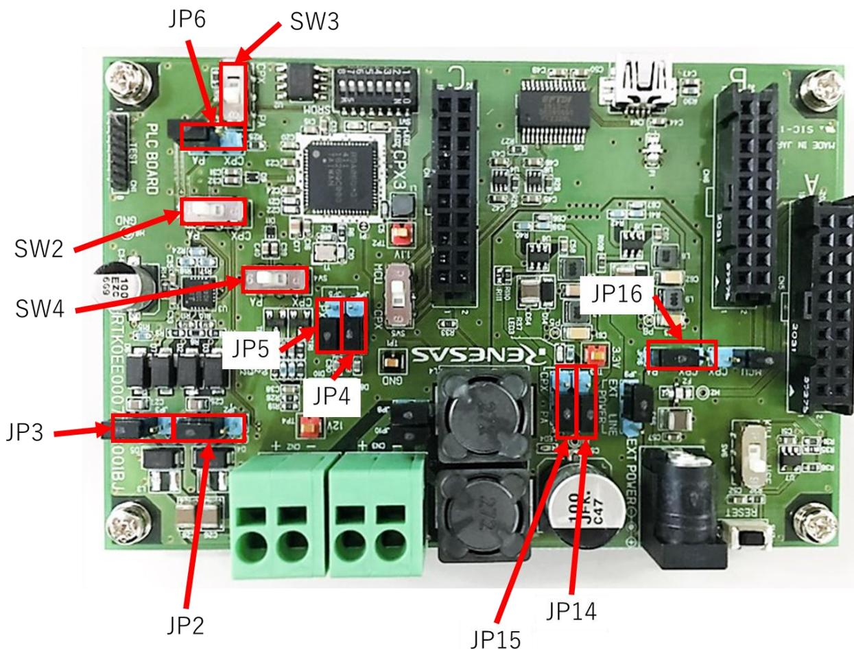
Figure 2-8 Setting parts for selecting drive system
