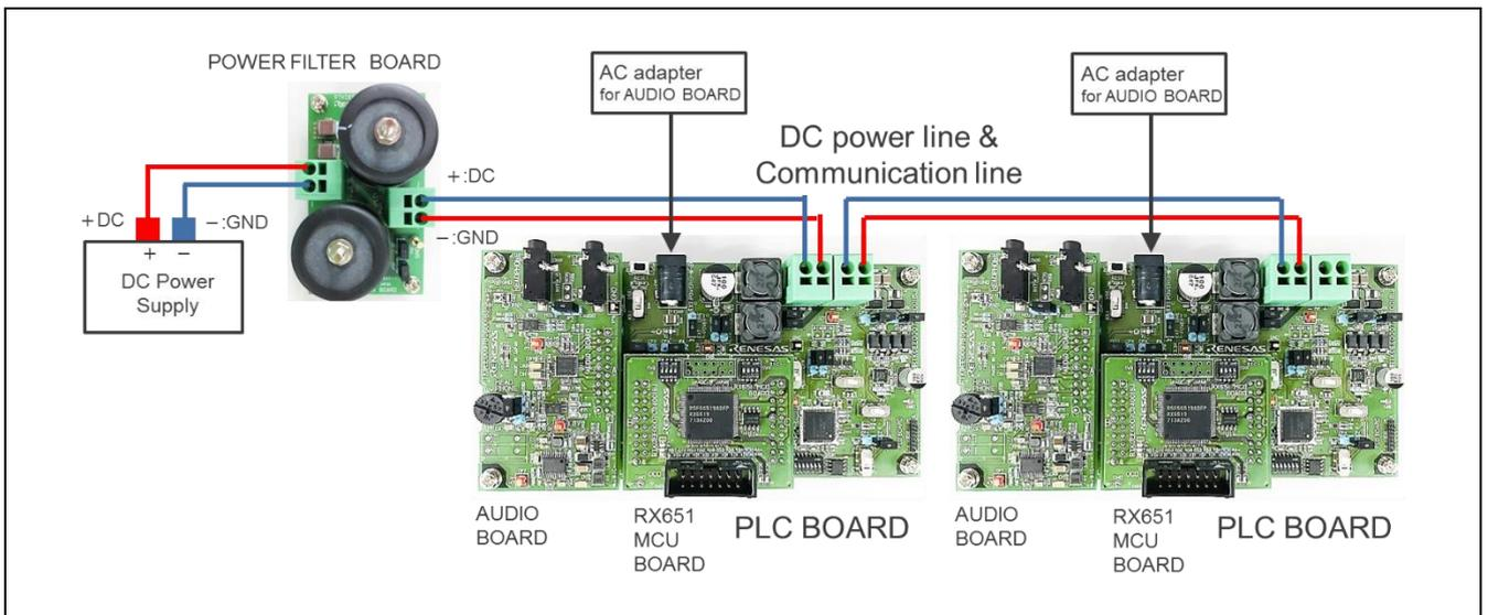
**Figure 2-7 Condition 6 : PLC board + RX651 MCU board + Audio board**
