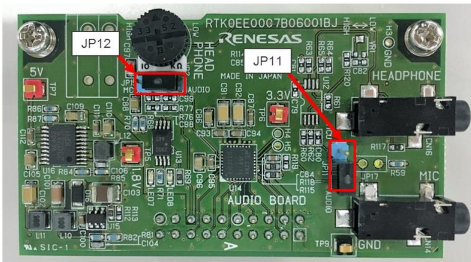
Figure 2-9 Audio board setting parts
