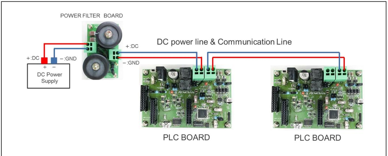
Figure 2-2 Condition 1: PC board connection example of DC power supply from the communication line
