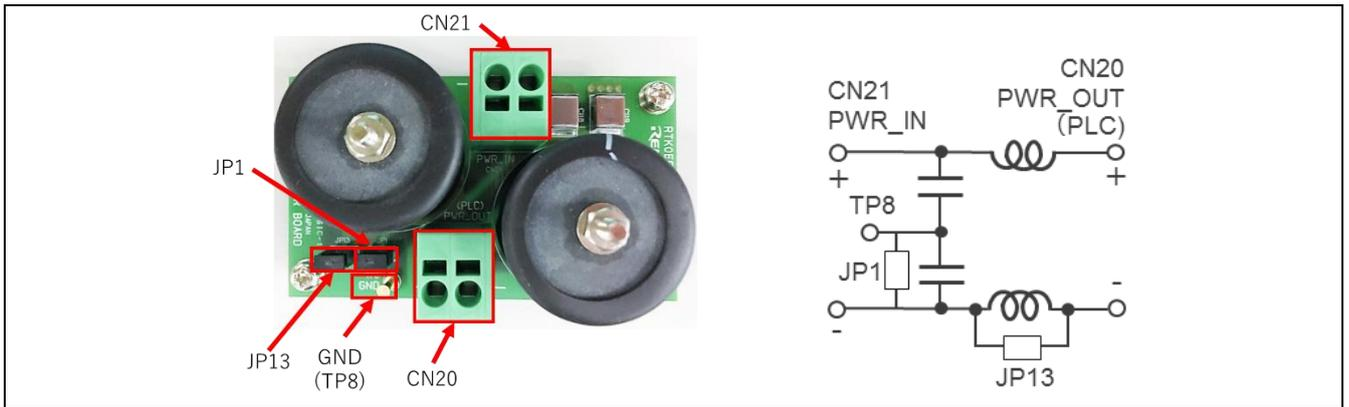
Figure 1-11 Power filter board connector, JP and TP
