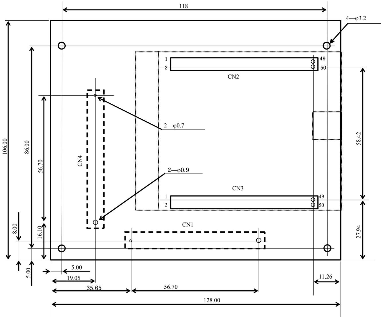
External Dimensions of M3A-ZA53 (Unit: mm) (1/1)
