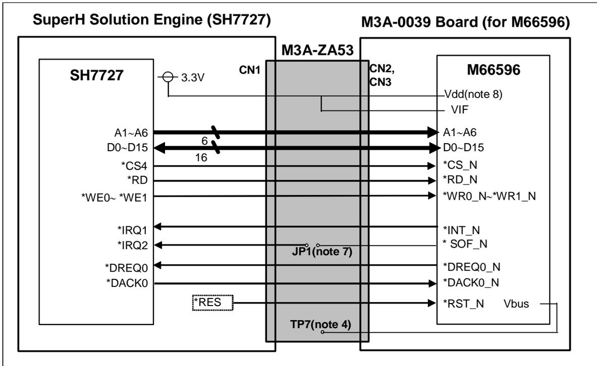
Figure 6.6 M3A-0039 (for M66596) and SuperH Solution Engine (SH7727)
