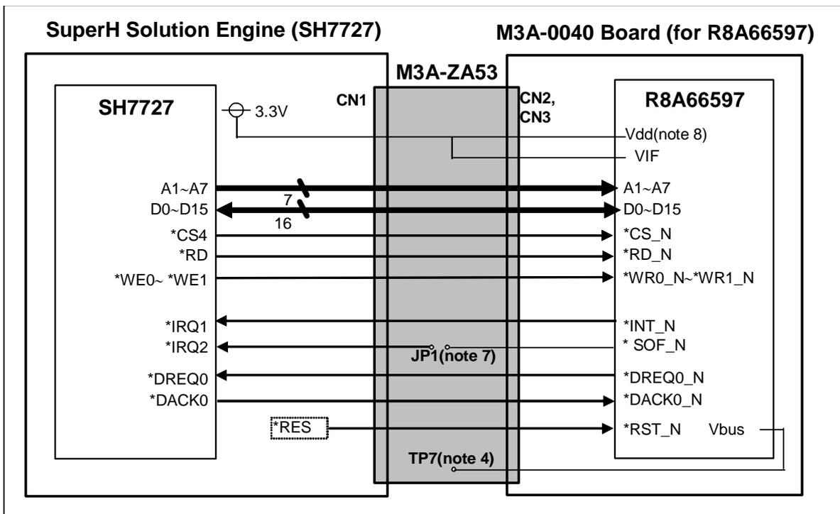
Figure 6.7 M3A-0040 (for R8A66597) and SuperH Solution Engine (SH7727)
