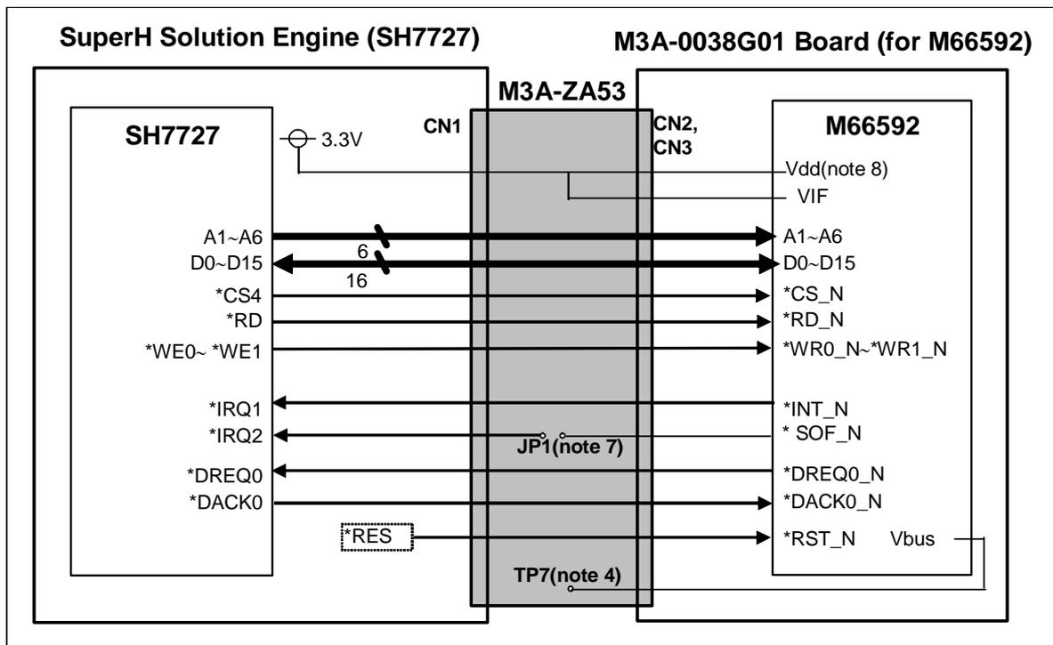
Figure 6.5 M3A-0038G01 (for M66592) and SuperH Solution Engine (SH7727)
