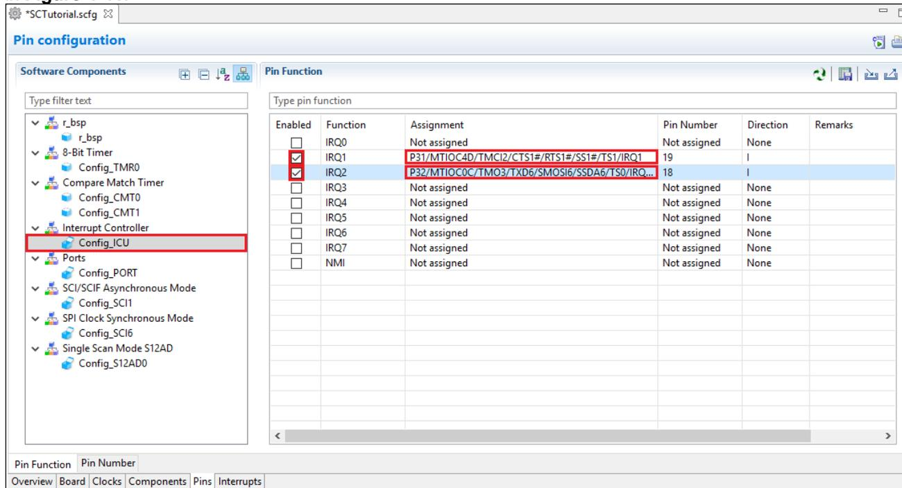
Figure 4-41 Configure pin assignment - Config\_ICU
