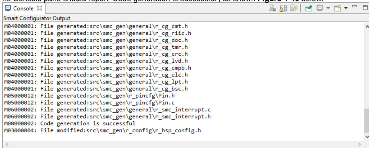
**Figure 4-46 Smart Configurator console**
