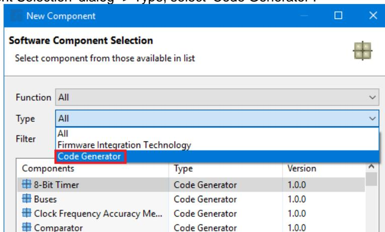
Figure 4-5 Add a Code Generator component (2)
