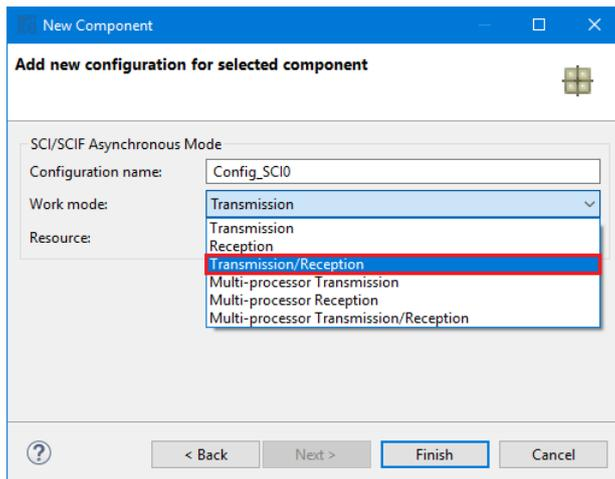
**Figure 4-26 Select Work mode – Transmission/Reception**
