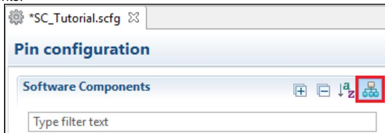
Figure 4-40 Change view to show by Software Components
