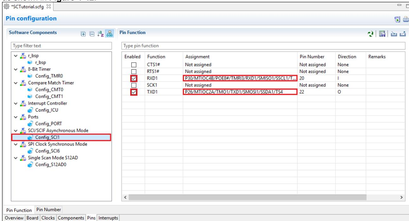
Figure 4-42 Configure pin assignment - Config\_SCI1
