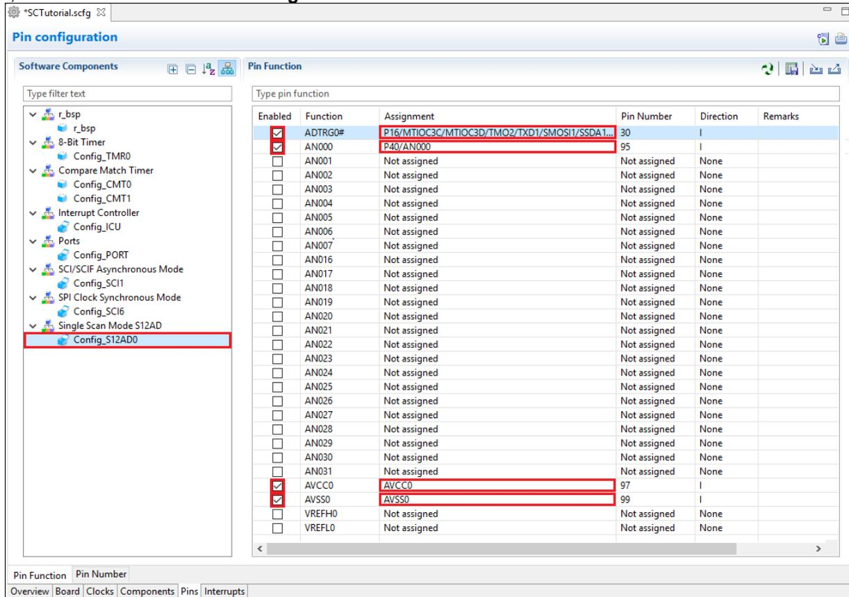
**Figure 4-44 Configure pin assignment - Config\_S12AD0**
