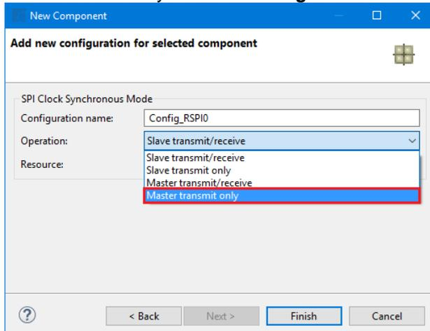
**Figure 4-31 Select Operation – Master Transmit**
