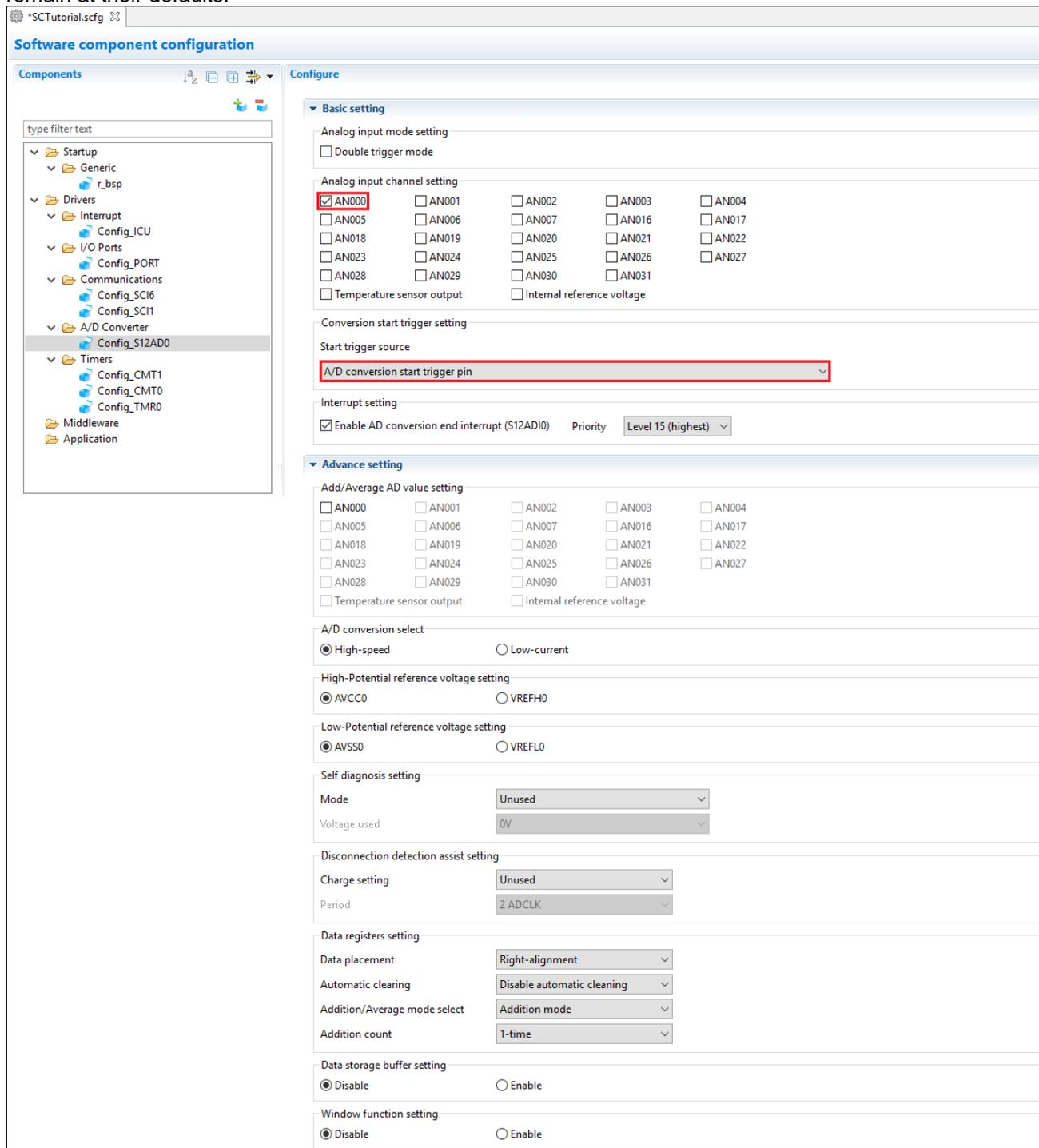
Figure 4-37 Config\_S12AD0 setting (1)
