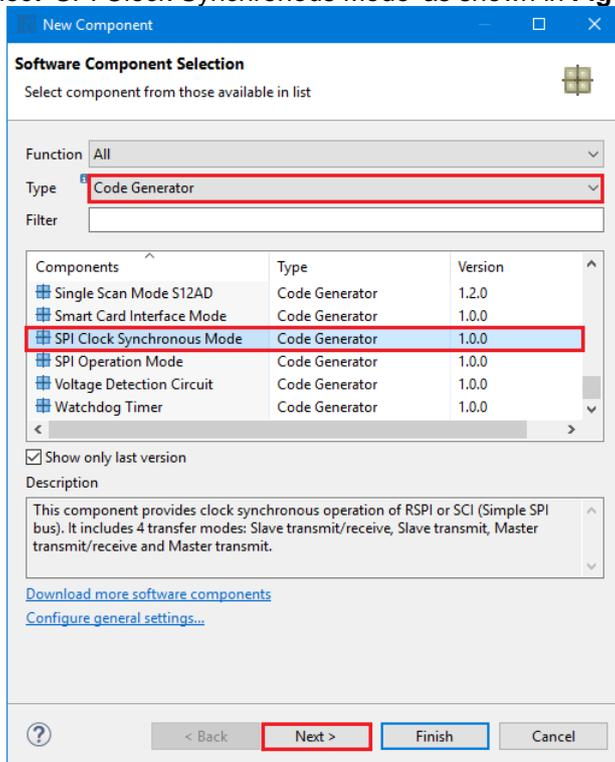
**Figure 4-30 Select SPI Clock Synchronous Mode**
