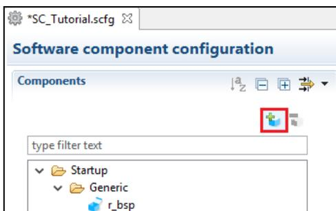
Figure 4-4 Add a Code Generator component (1)
