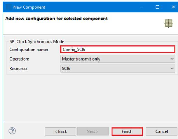
**Figure 4-33 Ensure Configuration name - Config\_SCI6**
