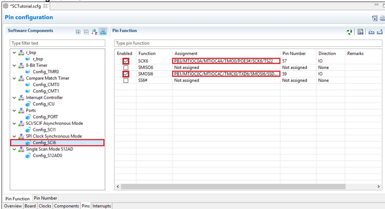
**Figure 4-43 Configure pin assignment - Config\_SCI6**
