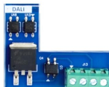
The DALI specification defines signal voltage levels that are much higher than the rest of the DK-S128. Circuitry on the DK-S128 provides the electrical interface needed to interface the DALI signal levels with the low voltage signal levels of the S128 MCU. Details of the electrical circuits can be found on page 6 of the electrical schematic. See Section **Error!** **Reference source not found..**
