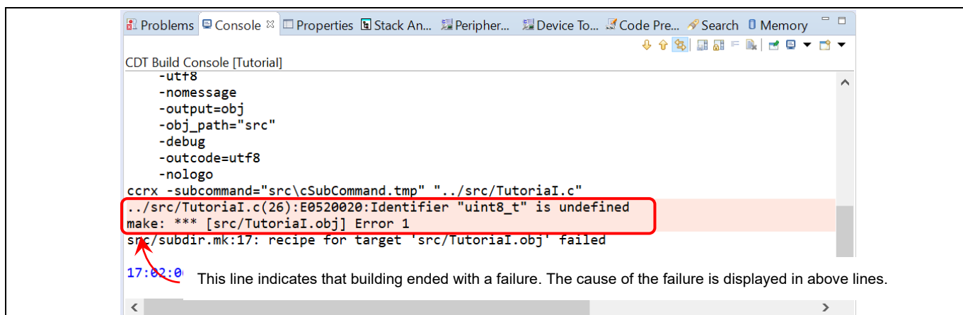
Figure 4-7 Unsuccessful Build Shows Error Messages
