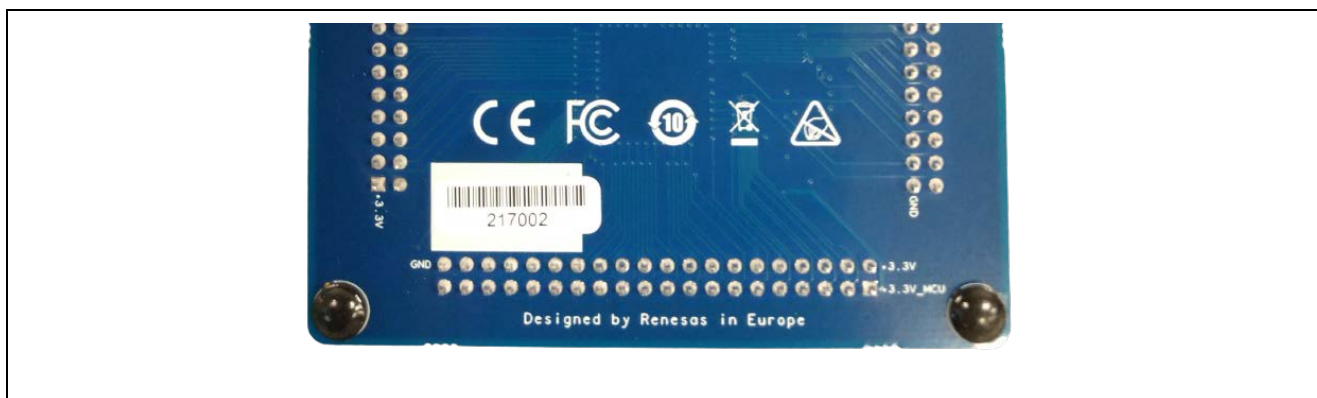
Figure 7. Identification of the Serial Number on the EK-RA2L1 Board
